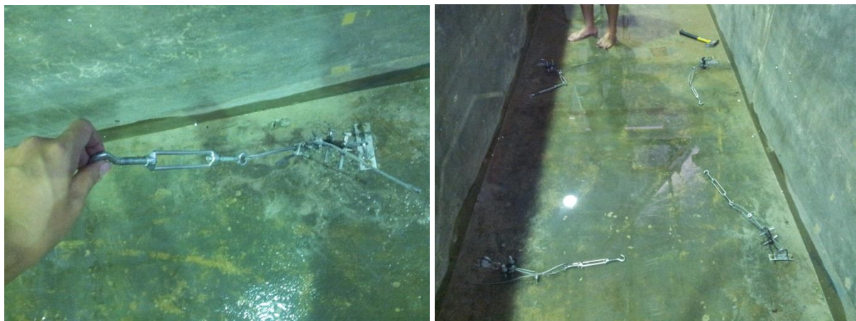
Figure 3.7: Mooring connection set up showing (a) mooring lines cable and (b) ground attachment points
