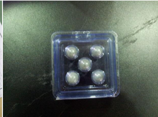
Figure 3.11: (a) Optical Tracking System camera, (b) reflective balls
