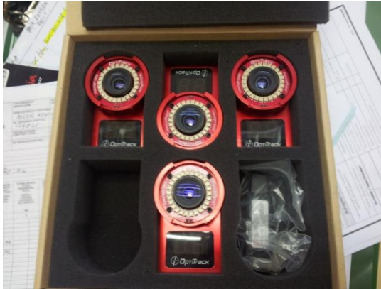
Figure 3.11: (a) Optical Tracking System camera, (b) reflective balls
