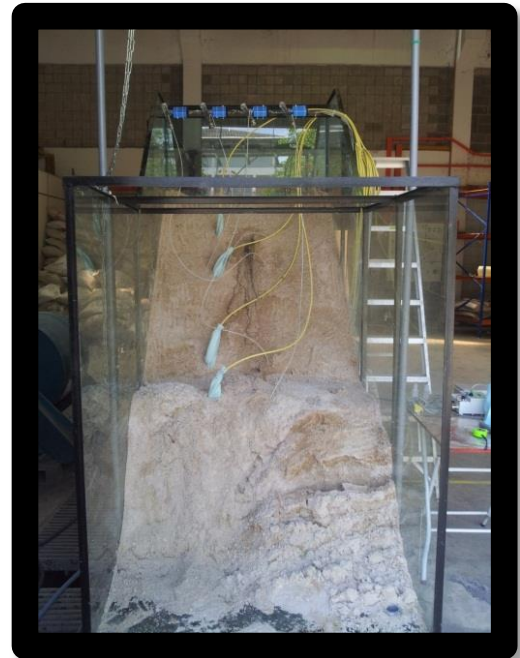
Figure 11 Installation of sensor devices
