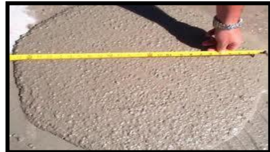
Figure 3.6: Slump flow and slump T_{50} test
