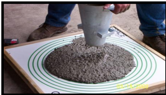
Figure 3.6: Slump flow and slump T_{50} test
