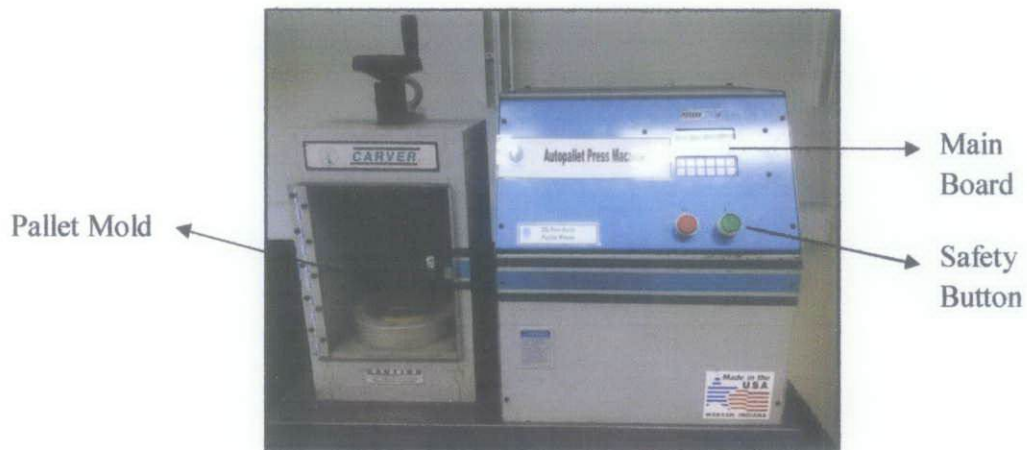
Figure 3.3: Auto pallet Press Machine
