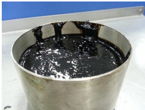
Figure 26 : Modified Binder with LDPE (after one day storage)
