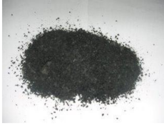
Figure 15 : Sieved rubber crumb
