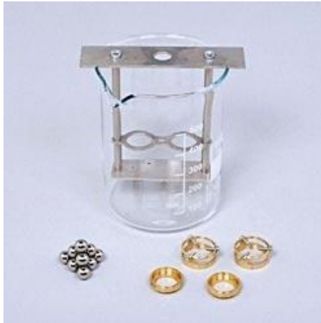
Figure 20 : Ring and Ball Apparatus
