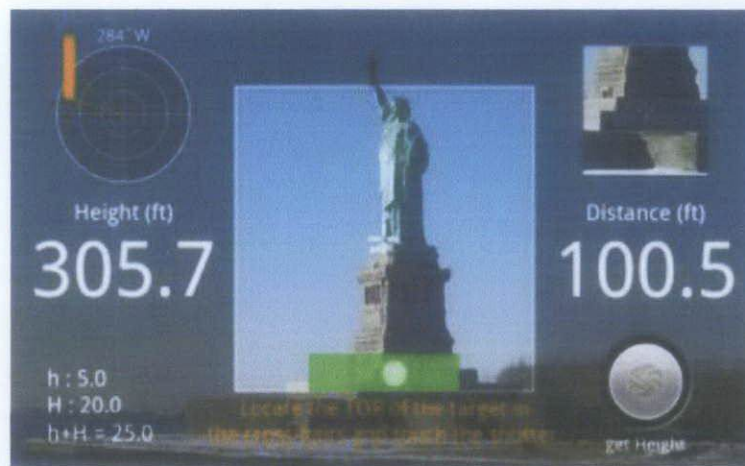
Figure 4: User will need to aim the cursor on the bottom of the object (as shown in the picture) and tilt the camera to get proper angle before capturing the image, in order for the application to calculate the distance.
