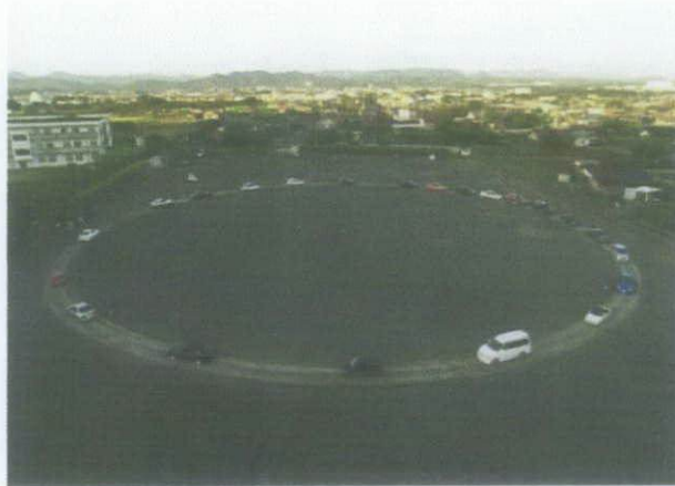
Figure 1: A snapshot of the experiment on a circular road. The circumference is 230 m, and the number of vehicles is 22. A 360-degree video camera is situated at the center of the circle for measurement [1].
