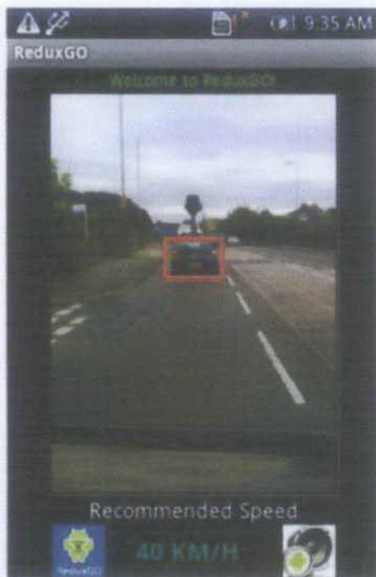
Image 1: ReduxGO detect car motion from the camera image. Based from the detection area, the application will recommend the appropriate speed for the driver in order to maintain safe distance between user's car and preceding vehicle.
