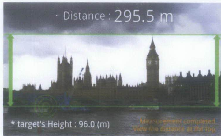
Figure 5: By using touch screen help, user will need to specify the target's range between two (2) horizontal lines, as shown in the Figure.
