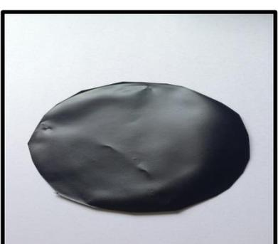
Figure 4-6: Ionic Liquid Mixed Matrix Membrane 4
