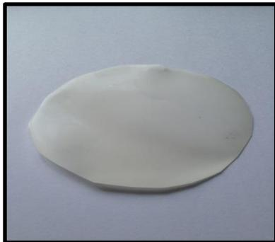
Figure 4-3: Ionic Liquid Mixed Matrix Membrane 1
