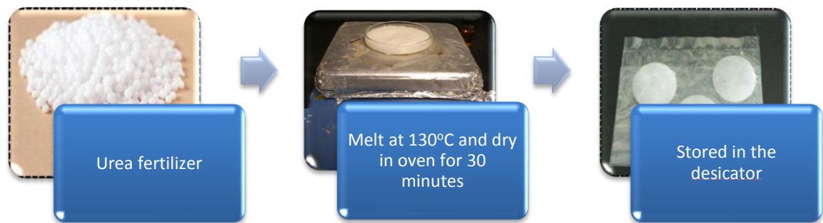
Figure 7 The flow diagram of urea substrate preparation
