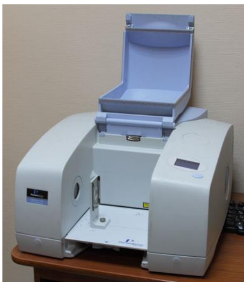
Figure A1: PerkinElmer FTIR Spectrometer
