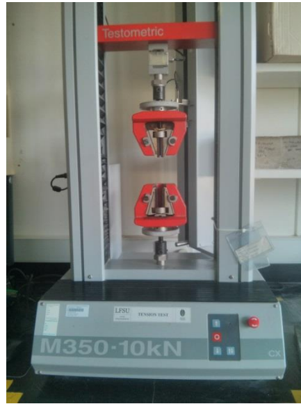
Figure A5: Testometric Tensile Tester
