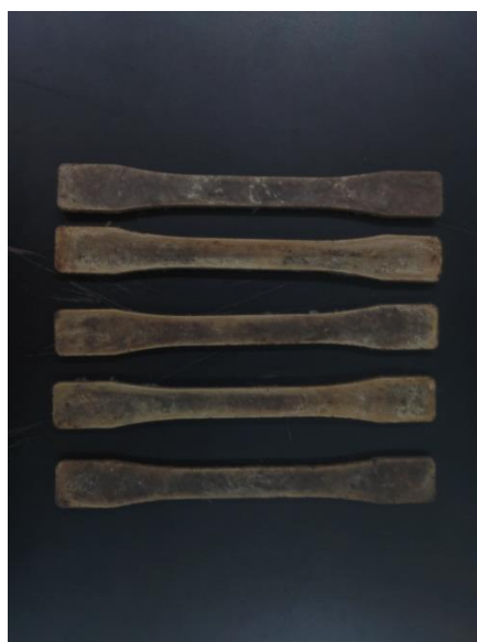
Figure A4: Dumbbell shaped sample specimen for tensile testing
