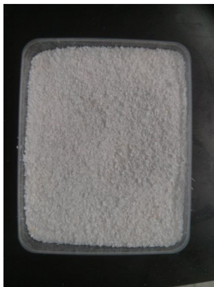
Figure A2: Recycled nylon precipitates grinded into powder
