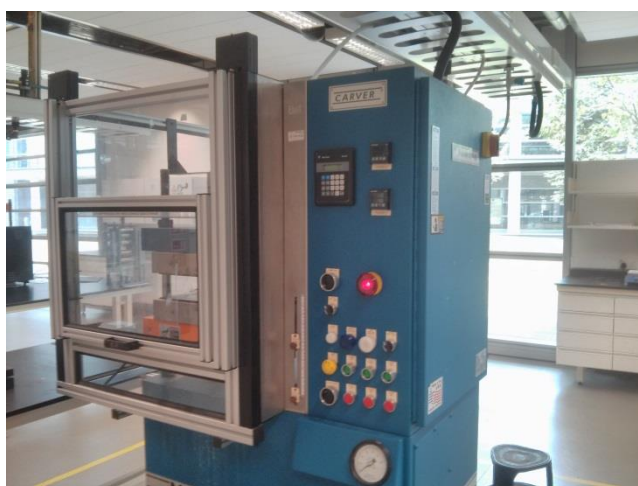
Figure A3: CARVER Compression Moulding Equipment
