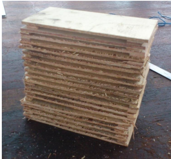
Figure 32 Stack of plywoods as packing material.
