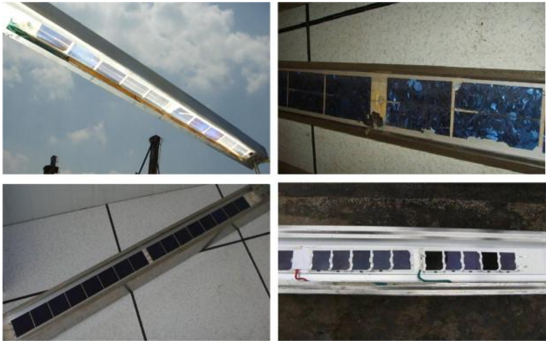
Figure 6 Four types of solar cell arrays, left top: single-crystalline silicon cell; right top: polycrystalline silicon cell; left bottom: Super cell; and right bottom: GaAs cell (L. G. L. Li M., Ji X., Yin F., Xu L., 2011).
