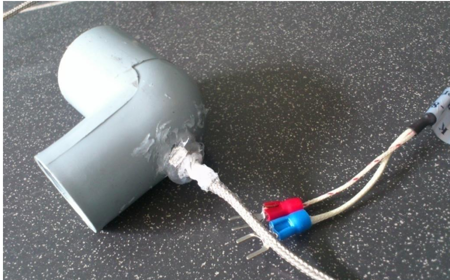
Figure 35 Thermocouple attached to inlet/outlet of the receiver by using silicon thermal compound and silicon glue.
