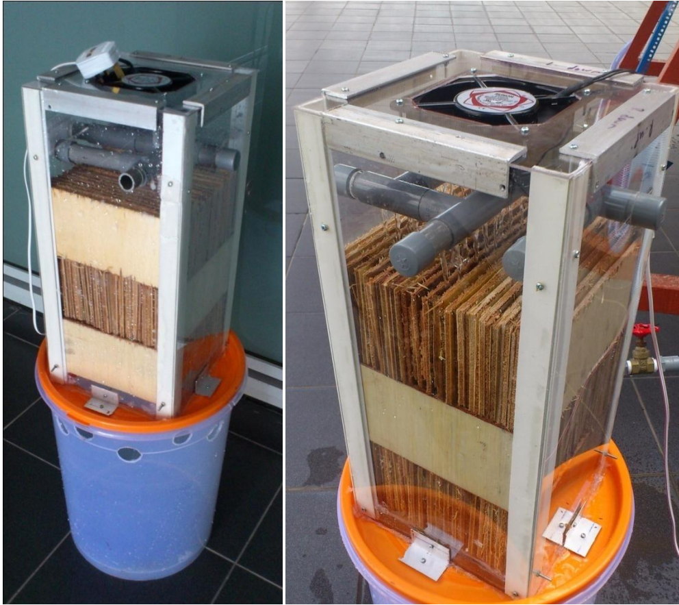
Figure 33 Left: The completed cooling tower placed on top of the water reservoir; Right: Cooling tower in action.
