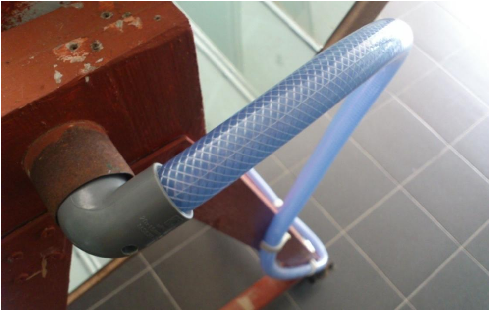
Figure 25 Close-up at the reinforced rubber tube. At the exit of the receiver, the tube was intentionally pointed upward to ensure that water fills up the receiver cavity.
