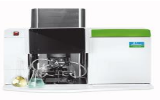
Figure 4: Atomic Absorption Spectrometry (Perkin Elmer AAnalyst 400)
