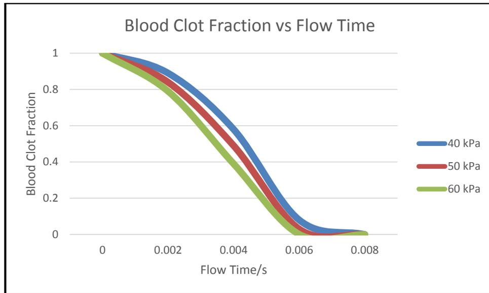
**Figure 18:** Graph of blood clot volume fraction against flow time under three phase model
