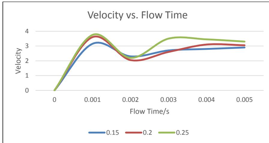
**Figure 16:** Grid Sensitivity Study under three phase model
