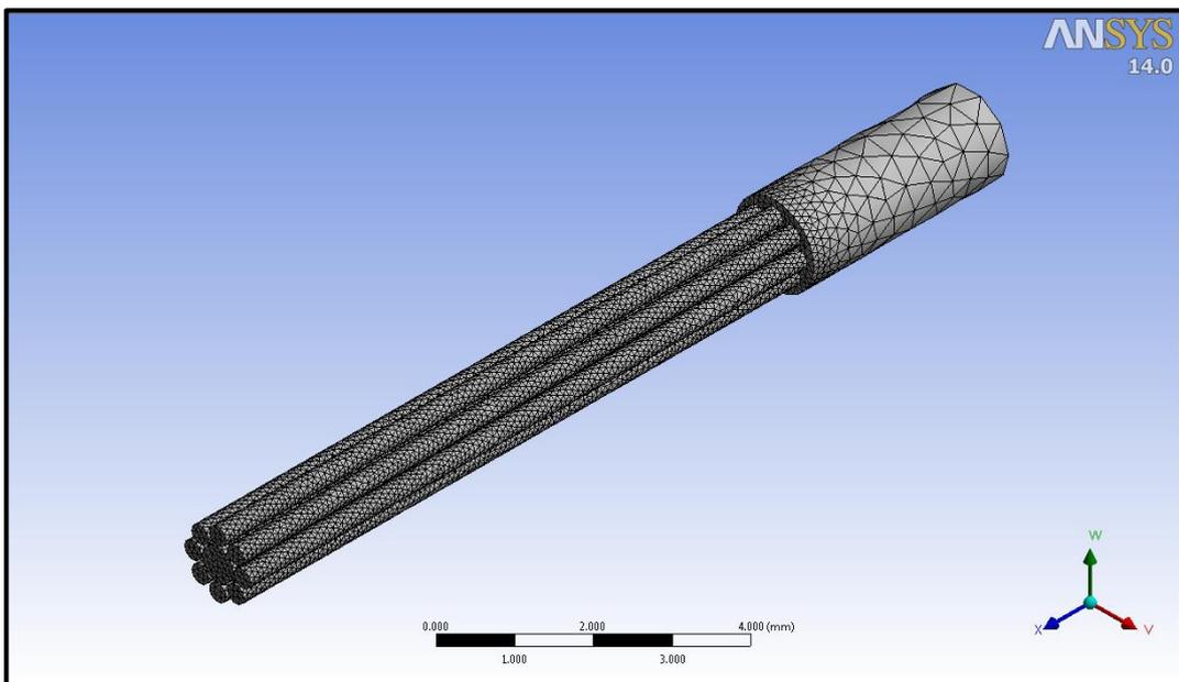
**Figure 15:** Meshed model of the new GP2 device (coarse)
