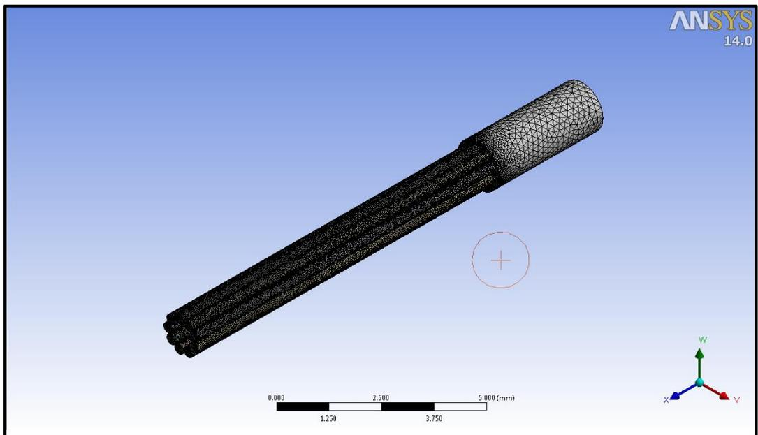
**Figure 12:** Meshed model of GP2 Device (coarse)
