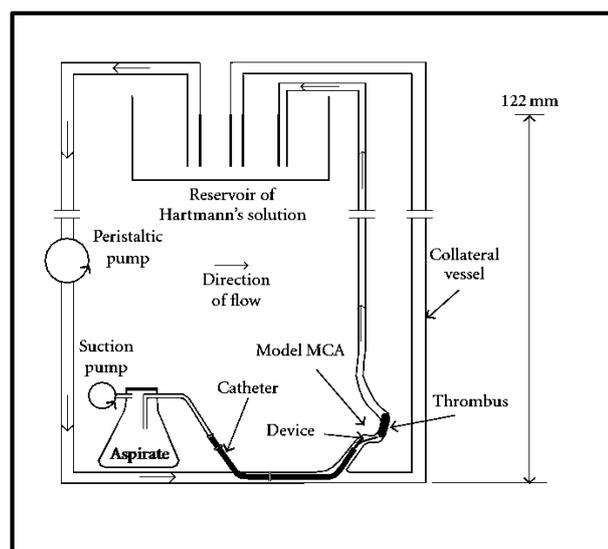
**Figure 6:** Pulsatile Flow System (Tennuci, et al., 2011)
