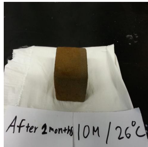
FIGURE 4.7 Geopolymer Sample (10M) after Immersed in Sulphuric Acid
