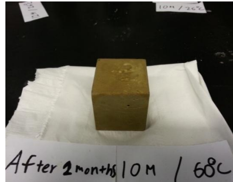
FIGURE 4.9 Geopolymer Sample (8M) after Immersed in Sulphuric Acid
