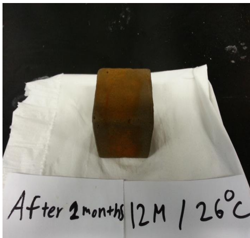
FIGURE 4.6 Geopolymer Sample (12M) after Immersed in Sulphuric Acid
