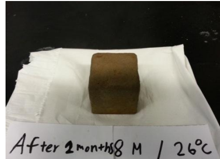
FIGURE 4.5 Geopolymer Sample (8M) after Immersed in Sulphuric Acid
