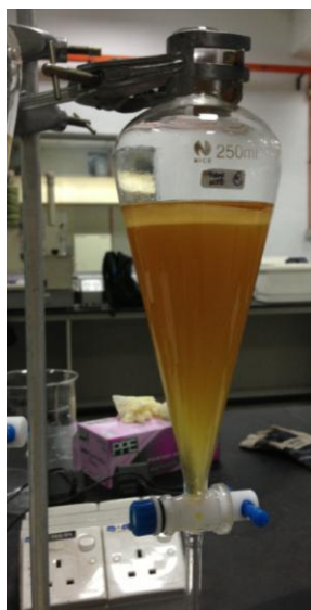
Figure 4.2: Separation of product and by-product layers after esterification
