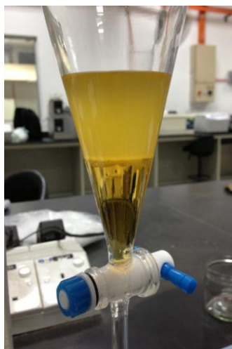
Figure 4.4: Separation of product and by-product layers after transesterification
