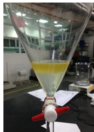
Figure 4.5: Washing of biodiesel after transesterification
