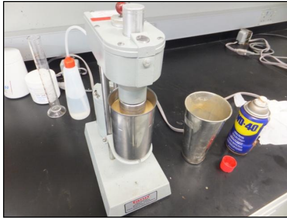
Figure 20: Mud Rheology Test Using Fann 35A Viscometer
