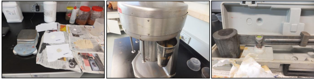
Figure 19: From L to R (Weighing additives for Mud Formulation, Mixing of Mud Using Fann multimixer, Mud Weight Test Using Mud Balance)
