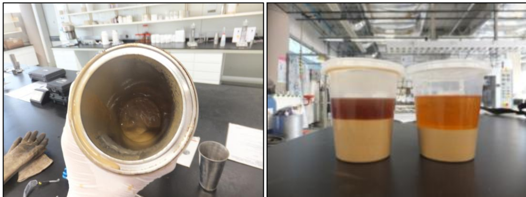
Figure 26: L-R: Clumping in the Aging Cell, Barite Sagging AHR and BHR
