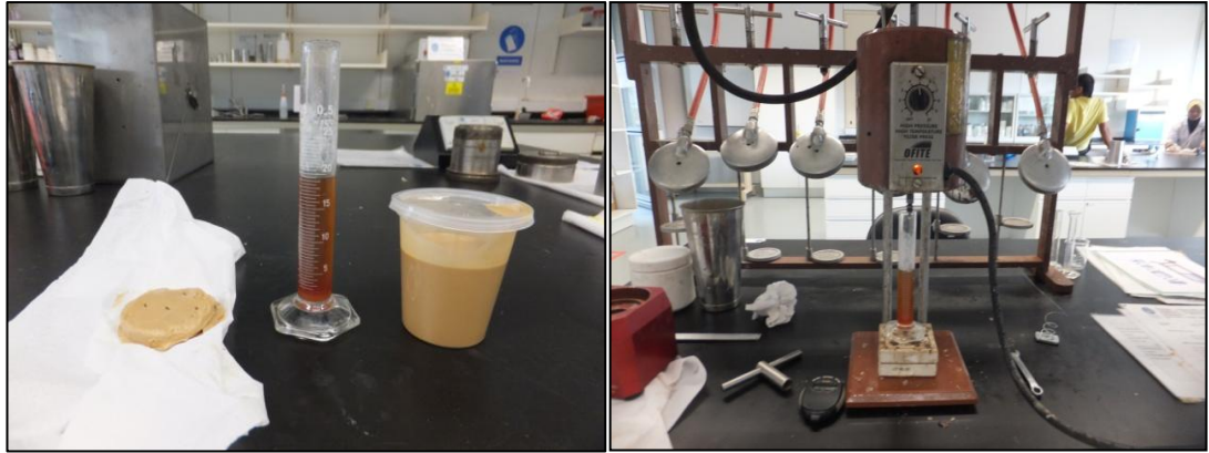
Figure 25: L-R: Mud Cake, Filtrate Loss, AHR Mud Sample, HPHT Filtrate Test
