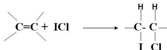
Figure 2-6 Double bond in fatty acid is reacted with iodine monochloride to produce di-halogenated single bond
