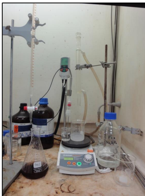
Figure 3-2 Apparatus set up for titration in Iodine Value Testing
