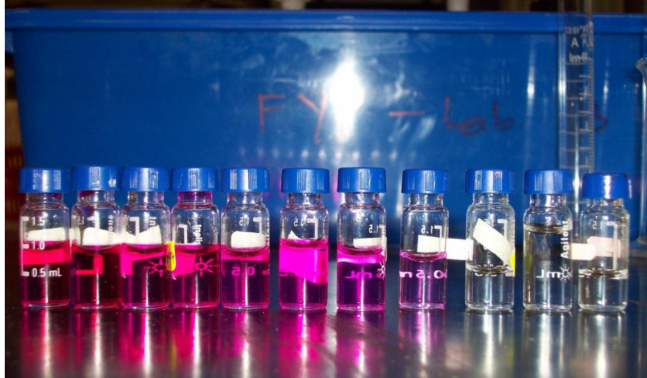
Figure 3.1.7: Phenol Dye Samples of Known Concentration
