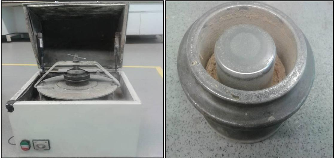
Figure 4.2: Grinding of dried rice husk using grinder.
