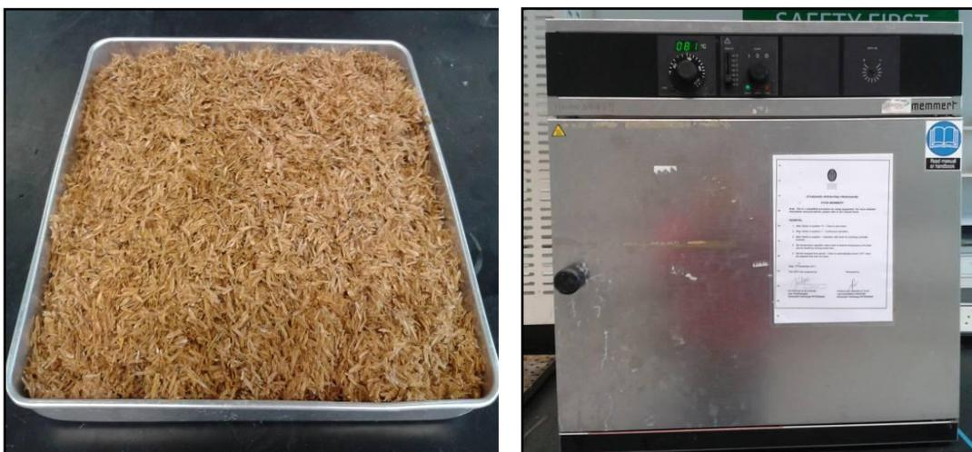
Figure 4.1: Cleaning and drying process of raw rice husk.
