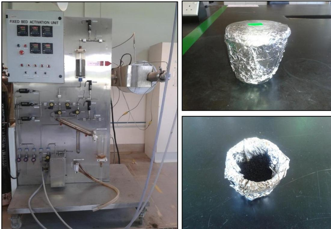
Figure 4.7: Fixed Bed Activation Unit and RHAC
