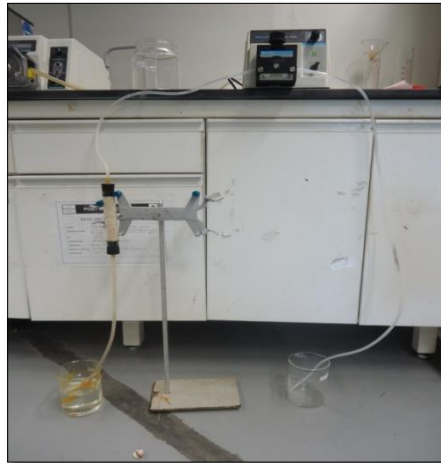
Figure 13 Experiment set up for continuous packed bed column
