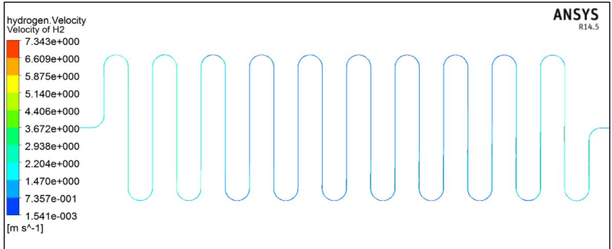
**FIGURE 4.6: Axial Velocity Contour of Hydrogen Gas Component**
