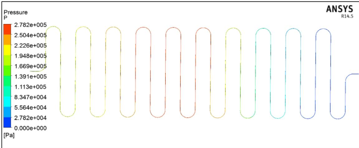
**FIGURE 4.10: Axial View of Pressure Difference across Microchannel**
