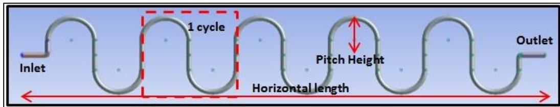
**FIGURE 2.6: Microreactor geometry (Rosli M. , 2012)**
