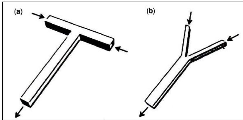
**FIGURE 2.1: (a) T-type and, (b) Y-type micromixers (Aubin & Xuereb, 2009)**
