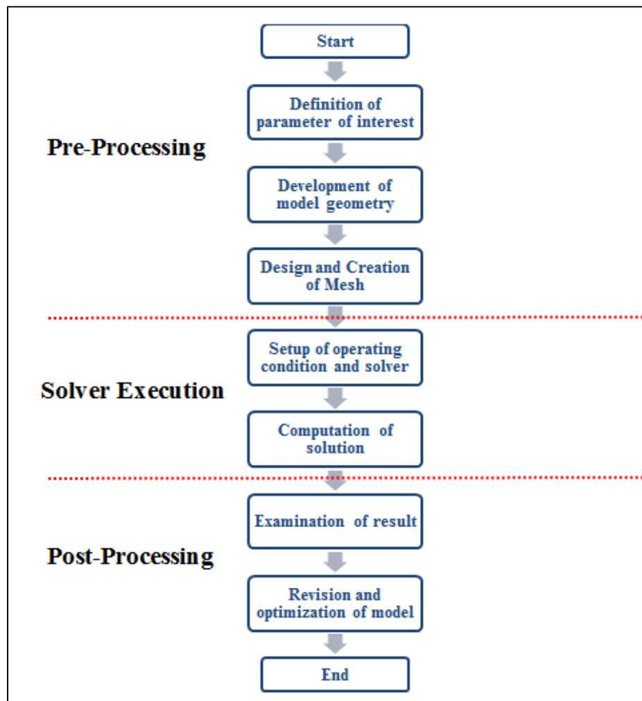
FIGURE 3.1: CFD Modeling Process Flow
