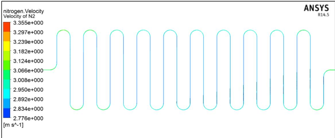
**FIGURE 4.8: Axial Velocity Contour of Nitrogen Gas Component**
