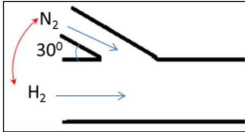
**FIGURE 2.7: Inlet geometry of 30° with hydrogen in the mainstream (Azeman M. K., 2012)**
