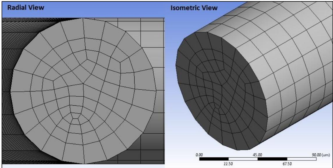
**FIGURE 4.2: Medium Meshing with 3,829,868 nodes**
