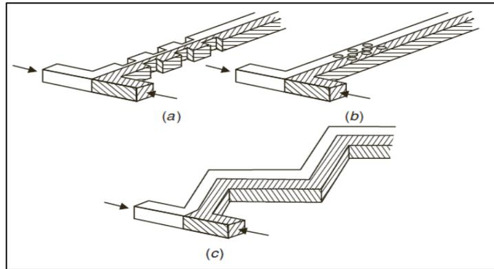
**FIGURE 2.2: Design for mixing with chaotic advection at high Reynolds numbers: (a) obstacles on wall (Wong, Ward, & Wharton, Micro T-mixer as a rapid mixing micro-mixer, 2004), (b) obstacles in the channel (Wang, Iovenitti, & Masood, 2002), (c) zigzag shaped channel (Mengeaud et al, 2002)**
