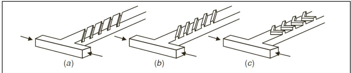
**FIGURE 2.3: Modification of mixing channel for chaotic advection at low Reynolds numbers: (a) Slanted ribs (b) Slanted grooves, (c) staggered-herringbone grooves. (Strook et al, 2002)**
