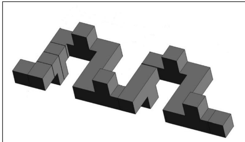
**FIGURE 2.4: Schematic of the micromixer proposed by Lin, Yu, Wang, Tu & Wang (2011)**
