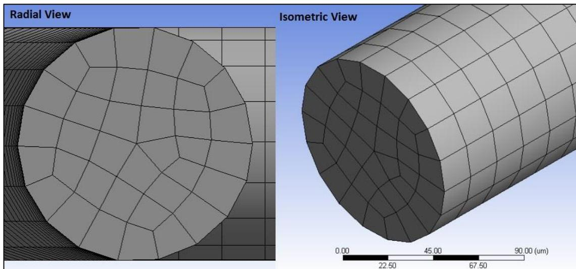
**FIGURE 4.1: Coarse Meshing with 3,704,981 nodes**
