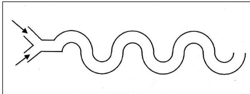
**FIGURE 2.5: Micromixer based on viscoelastic instability.(Nguyen, 2008)**
