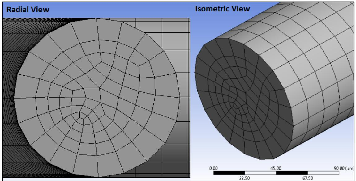
**FIGURE 4.3: Fine Meshing with 4,162,900 nodes**
