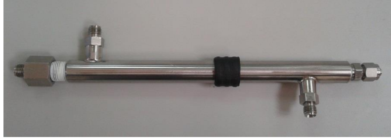
Figure 11: The lab-scale hollow fiber membrane module structure
