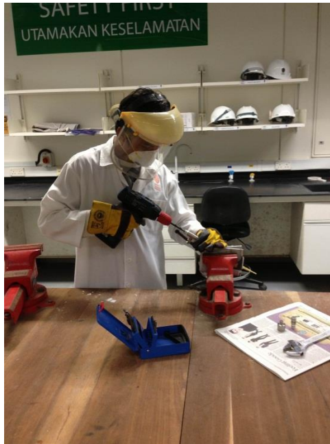
Figure 14: Removing solidified epoxy resin using hand drill
