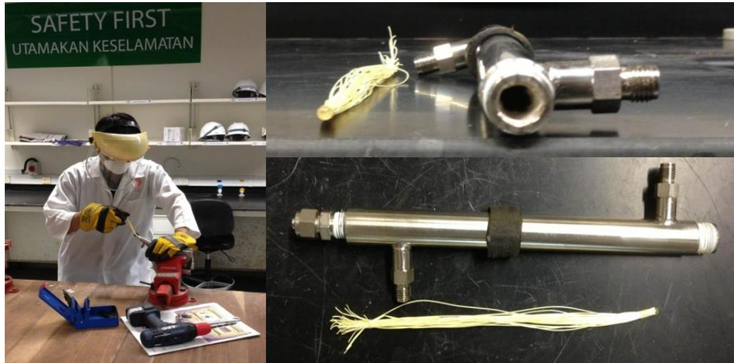
Figure 8: Membrane fiber potting
