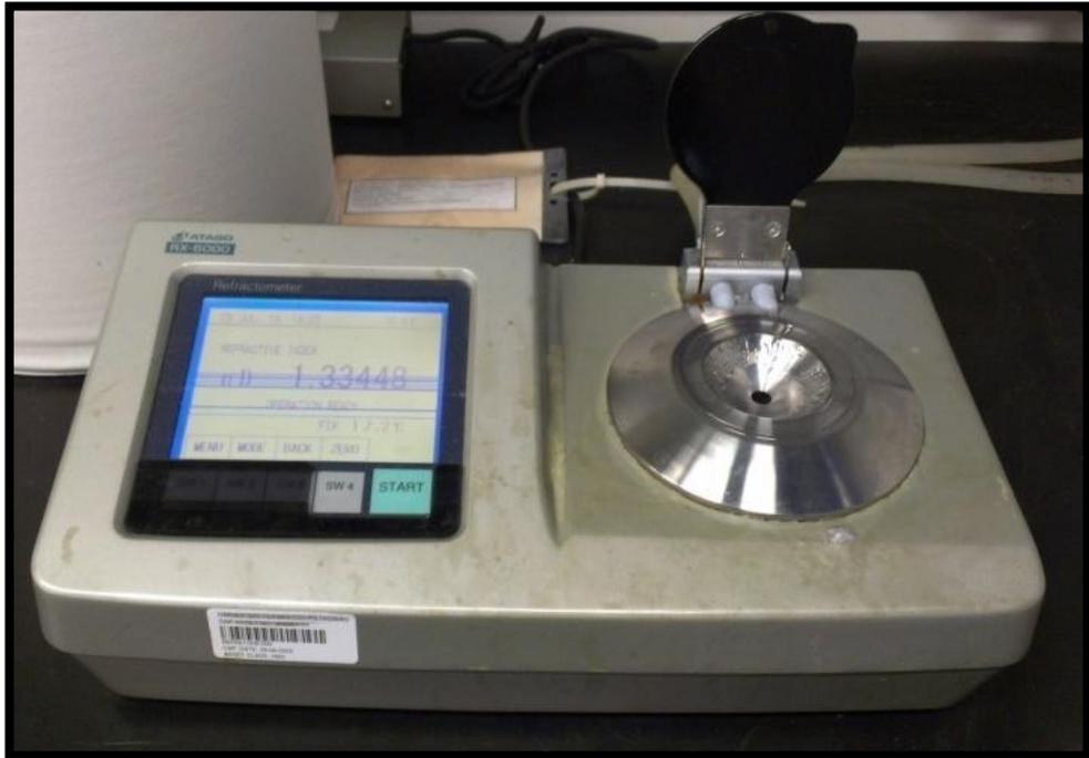
Figure 6 : Refractometer to measure refractive index
