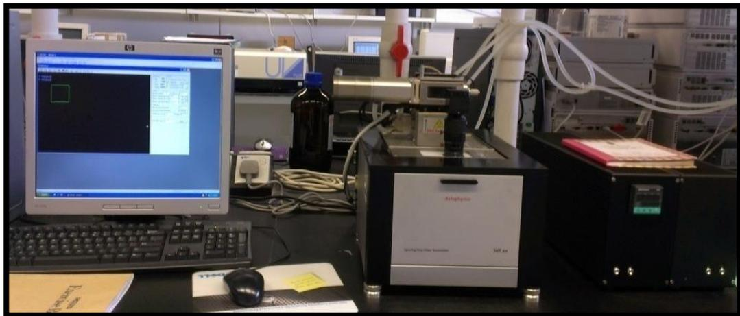
Figure 7 : Spinning drop tensiometer to measure interfacial tension
