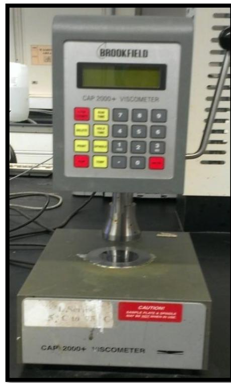
Figure 8 : Viscometer to measure viscosity
