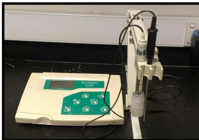
Figure 10 : pH meter to measure the pH value
