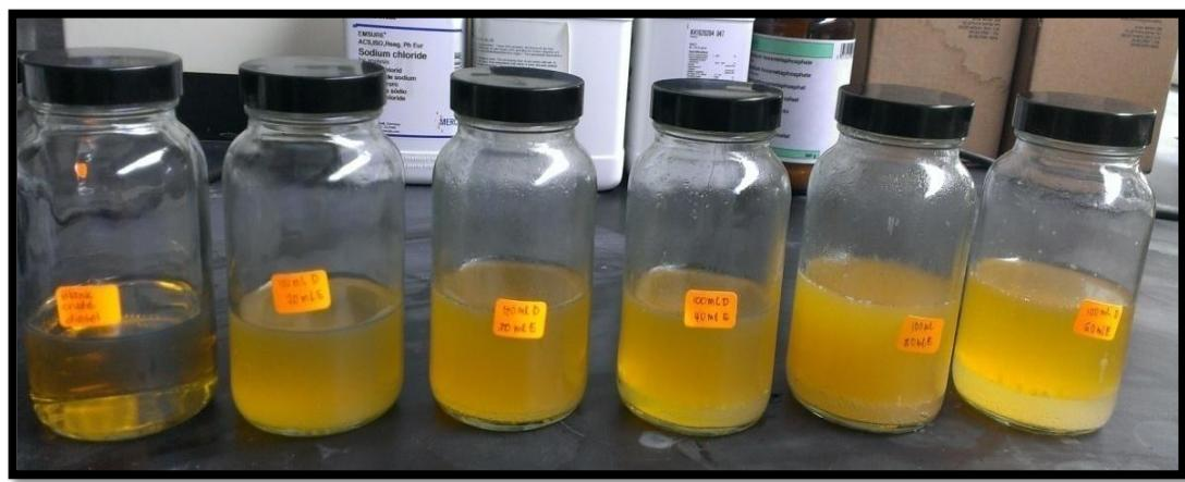
Figure 20 : Result of varying volume of emulsifier in 100 ml crude diesel
