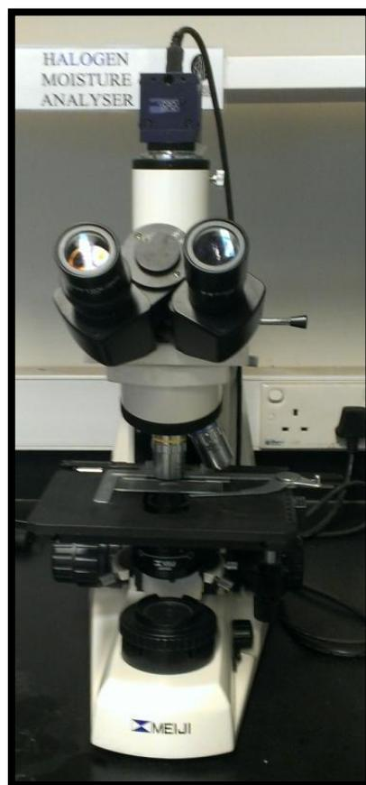
Figure 9 : Microscope to measure droplet size
