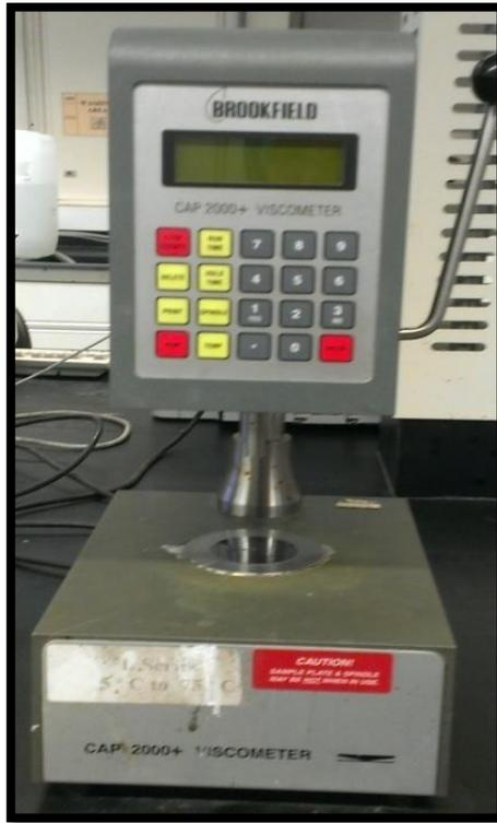
Figure 8 : Viscometer to measure viscosity
