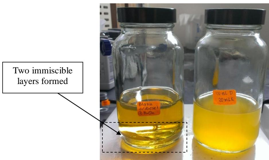
**Figure 14 : Different between crude oil with hydrogen peroxide (left) and emulsified crude oil (right)**
