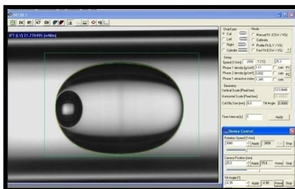
Figure 11 : Interfacial Tension Result for H<sub>2</sub>O<sub>2</sub>/Diesel
