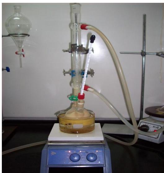
Figure 7: Soxhlet extractor available in laboratory [17]
