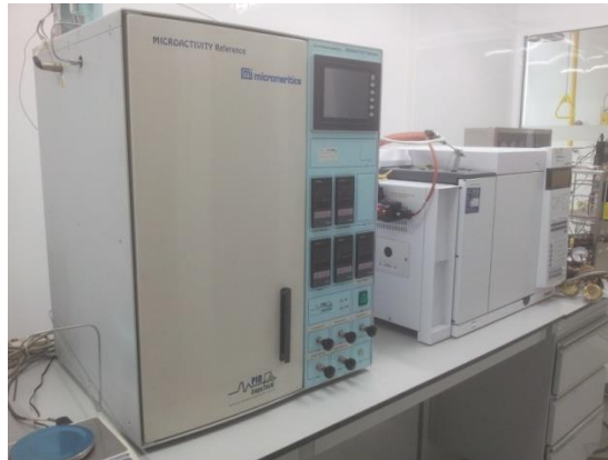
FIGURE 8. MICROACTIVITY-References connected to GC
