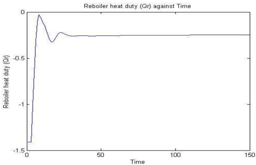
**Figure 16: Reboiler heat duty in deviation variable required for  $T_d$  set point change**
