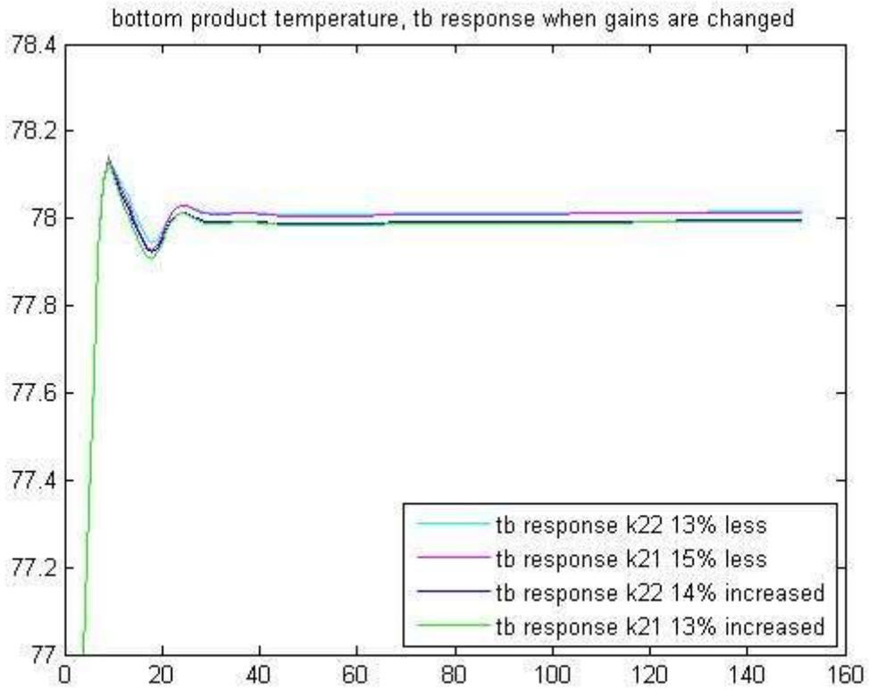
**Figure 20:  $T_b$  response when process gains increased and decreased**
