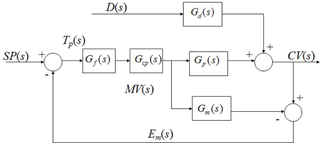
**Figure 3: Filter is added to model based predictive control**
