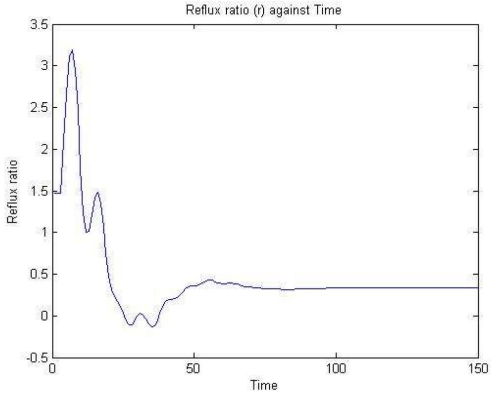
**Figure 11: Reflux ratio in deviation variable required for  $T_d$  set point change**
