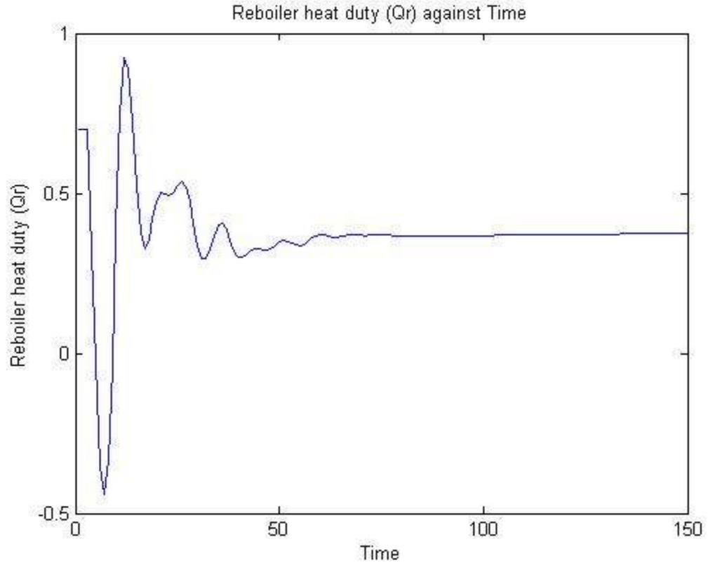
**Figure 12: Reboiler heat duty in deviation variable required for  $T_d$  set point change**
