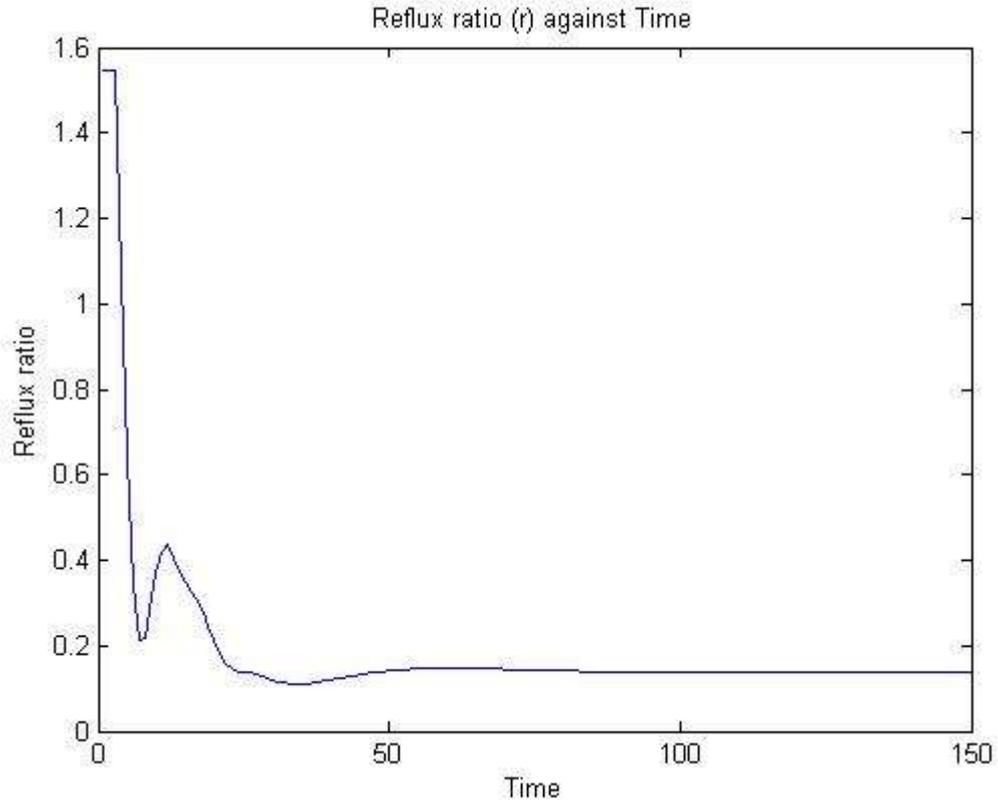
**Figure 15: Reflux ratio in deviation variable required for  $T_b$  set point change**
