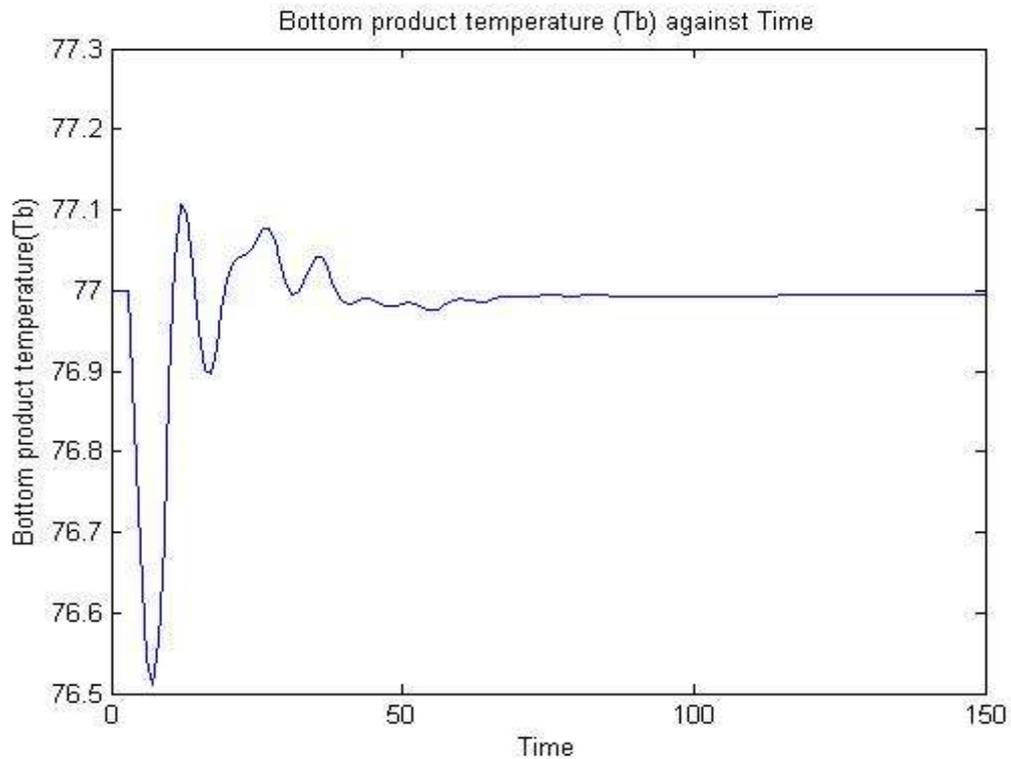
**Figure 10: Bottom product temperature,  $T_b$  response to  $T_d$  set point change**
