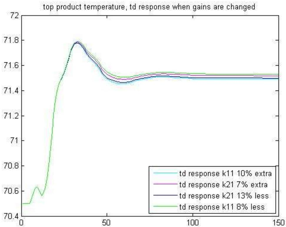
Figure 17:  $T_d$  response when process gains are increased and decreased
