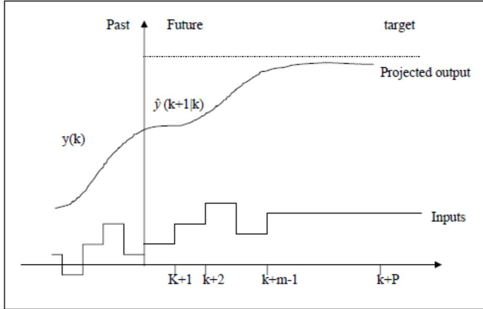
**Figure 2: Graph showing the projected output and inputs into the process**
