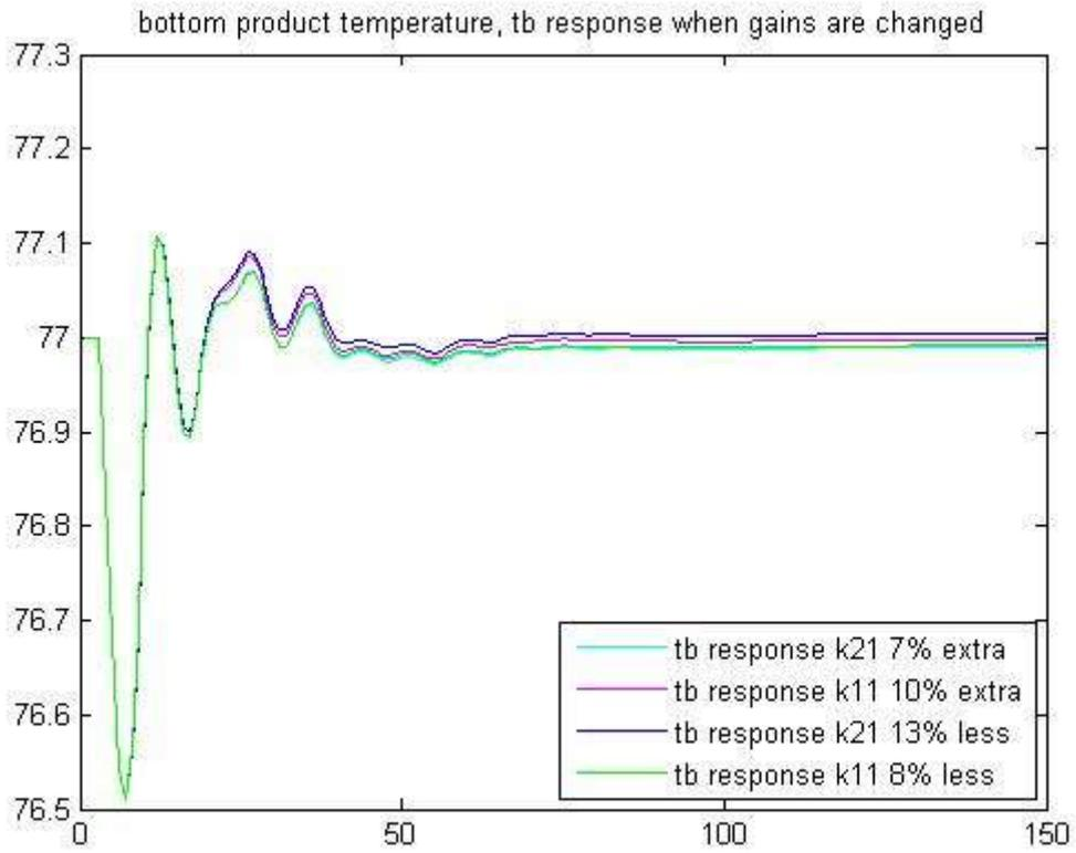
**Figure 18:  $T_b$  response when process gains are increased and decreased**
