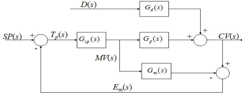
**Figure 1: Block diagram of model based predictive control strategy**
