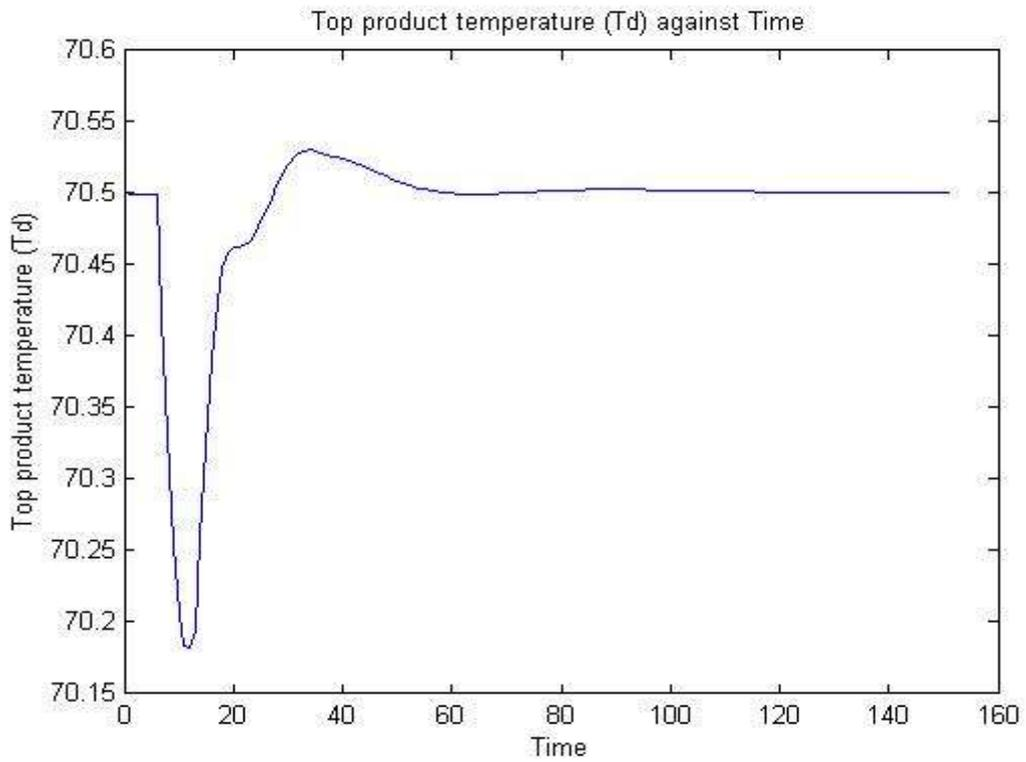
**Figure 13: Top product temperature,  $T_d$  response to its set point change**
