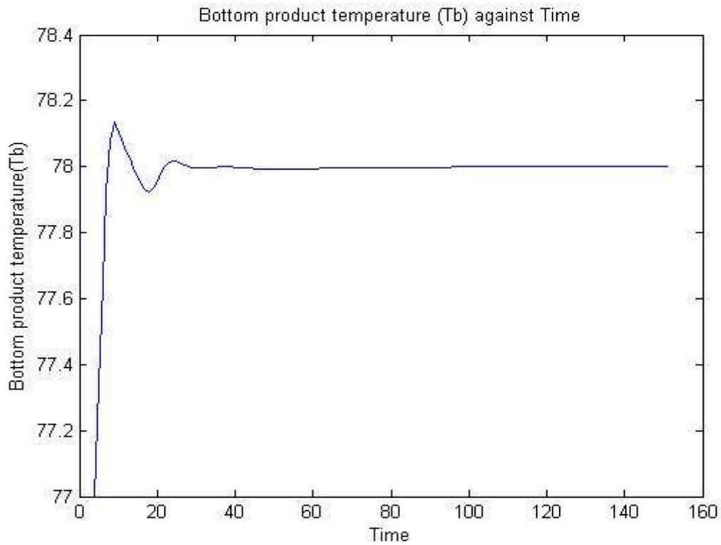
**Figure 14: Bottom product temperature,  $T_b$  response to its set point change**
