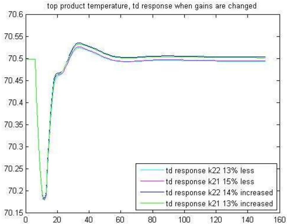
**Figure 19:  $T_d$  response when process gains increased and decreased**
