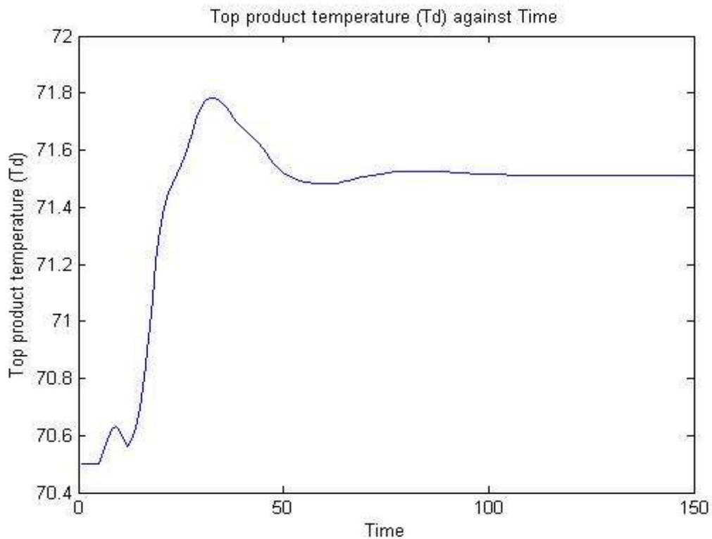
**Figure 9: Top product temperature,  $T_d$  response to its set point change**
