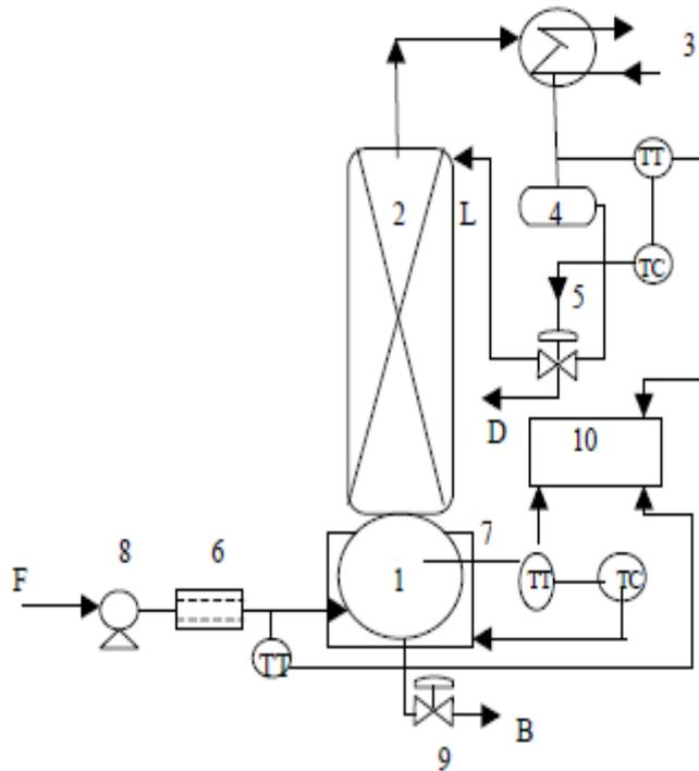
**Figure 5: Distillation column and equipments involve**
