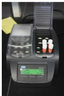
Figure 3.2.5.6 Digestion of COD samples in HACH DRB 200 digester
