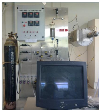
Figure 10 : Fixed Bed Activation Unit
