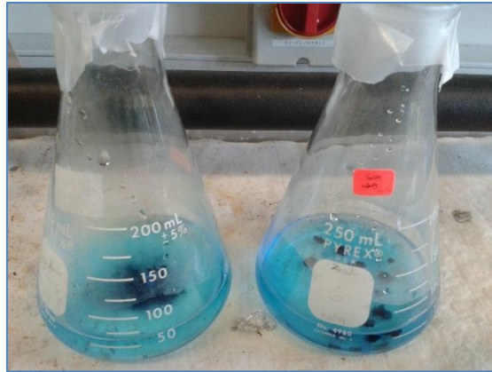
Figure 17 : Adsorption of methylene blue using durian shells activated carbon
