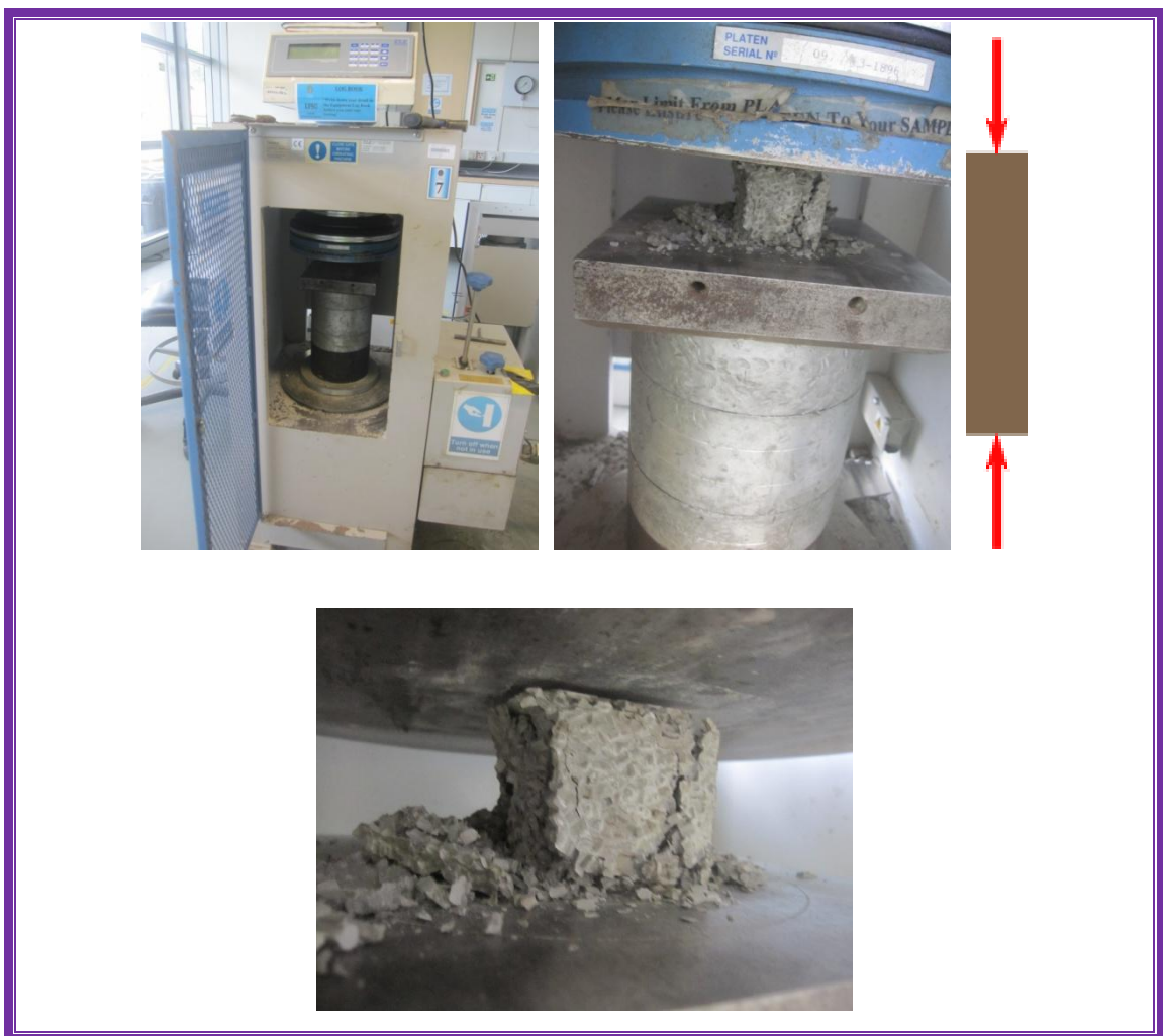
Figure 4.5: Compressibility Test. Top left: Compression Machine. Top middle: Sample tested inside compression machine. Top right: the direction of the compression with respective to the sample. Bottom: Sample crushed after testing.
