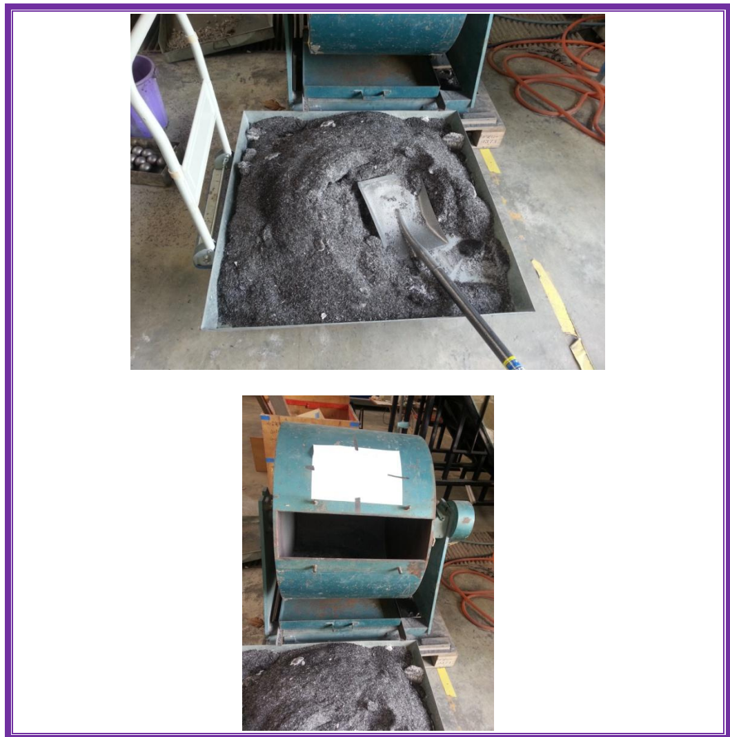
Figure 3.3: Preparation of RHA: RHA after taking out from the incinerator (photo above). RHA ready to put inside the ball-mill grinder (photo below).
