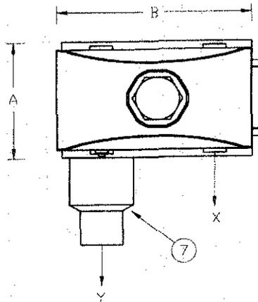
Figure 11: Design width =  $B = 67.7$  mm
