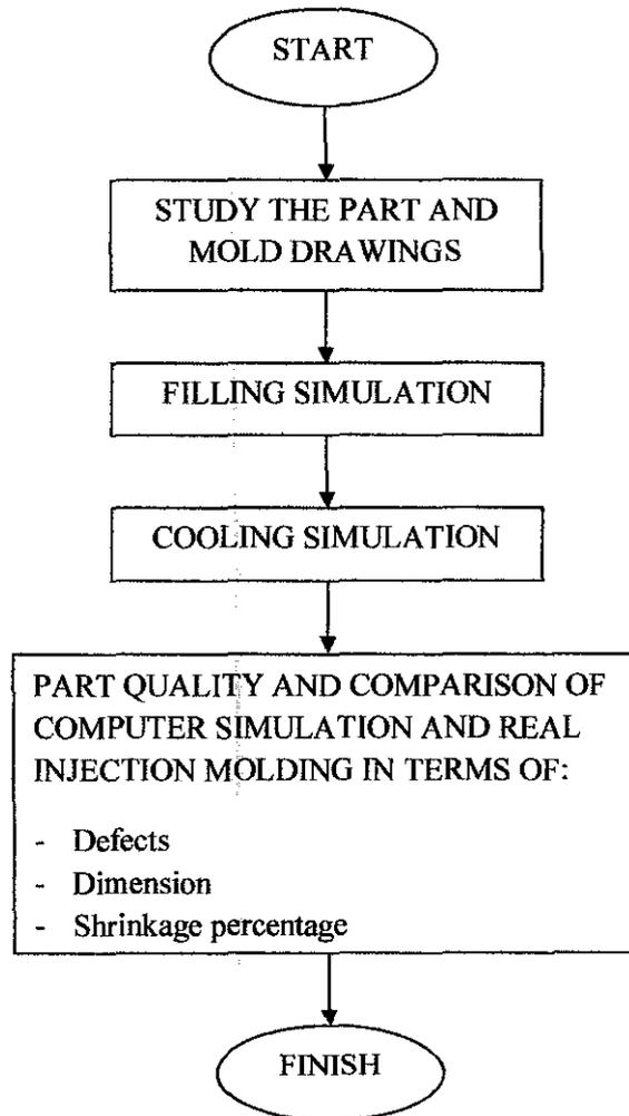
Figure 1: Methods used in simulation of injection molding for insulated piercing connector (IPC)
