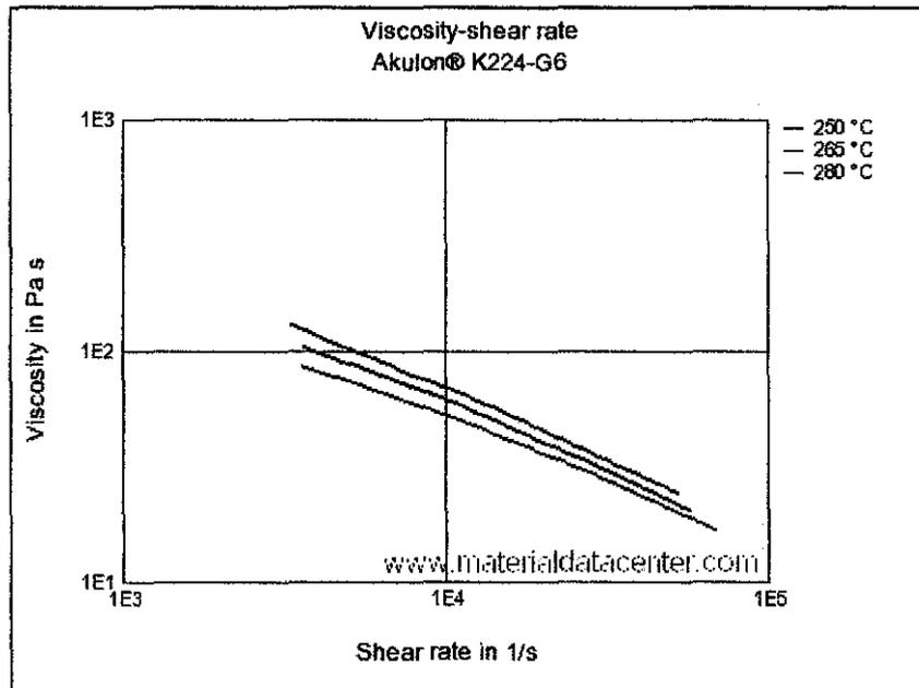
Figure 2: Viscosity versus shear rate graph[14]
