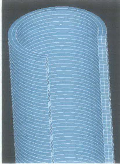
Figure 3.3: Element in \frac{3}{4} expansion of 2D axisymmetric model
