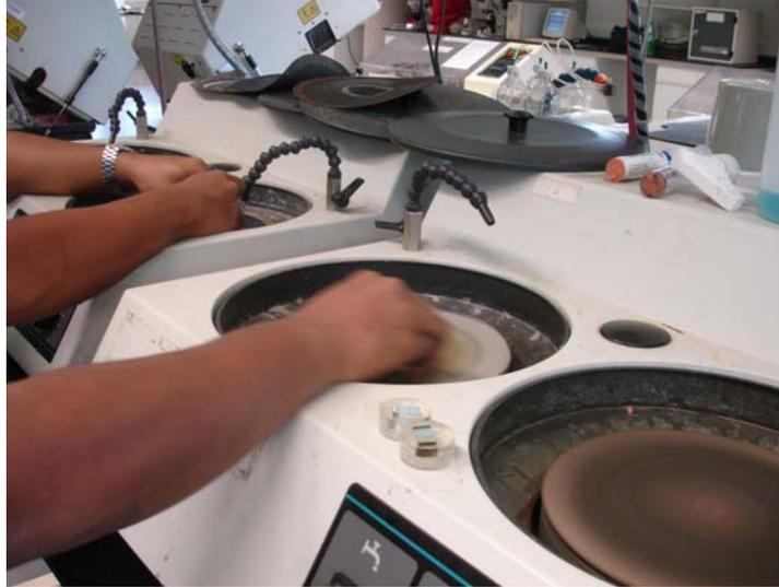
Figure 3.5 : Grinding and Polishing Process
