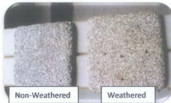
Figure 8: Example of colour comparison between non-weathered and weathered coatings
