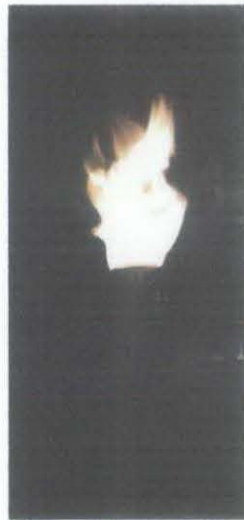
Figure 4.5: Flare produced from sugarcane bagasse gasification
