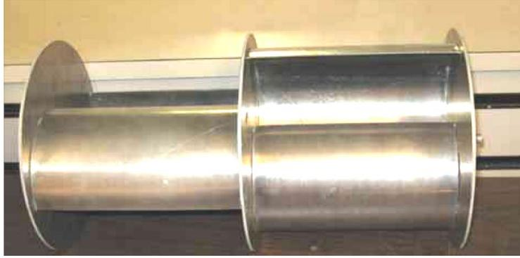
Figure 2.10: Double stage Savonius rotor
