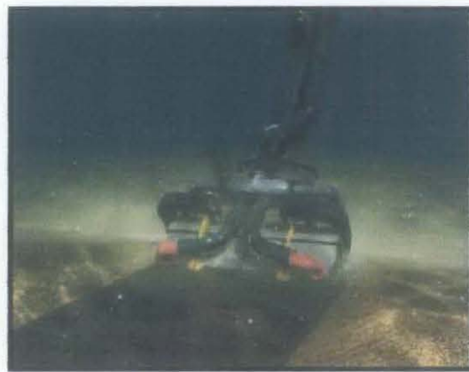
Figure 2.1: Drag head of a TSHD (Van Oord, 2010)
