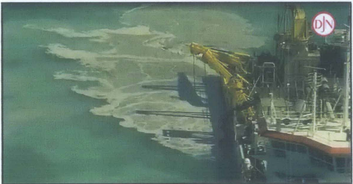
Figure 1.1: Overspills from Trailing Suction Hopper Dredger. (Jan De Nul, 2009)
