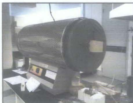
Figure 3.12: Carbolite horizontal furnace tube
