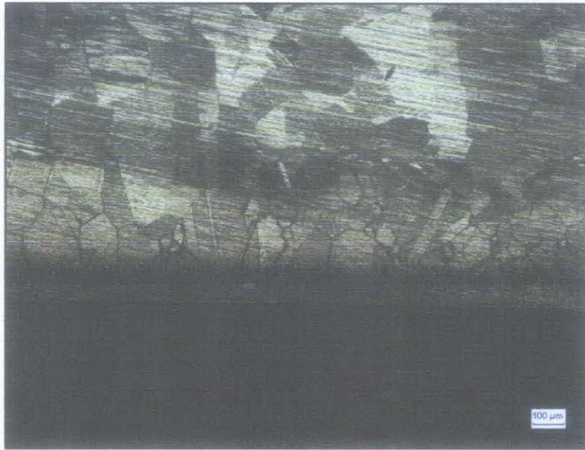
Figure 4.5: Microstructure of AISI 410 nitriding at 1050°C (under optical microscope).
