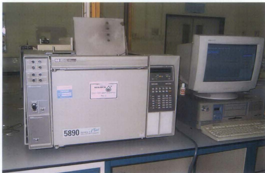
Figure 3.5 HP 5890 Series II High Temperature Gas Chromatography (HTGC) equipment
