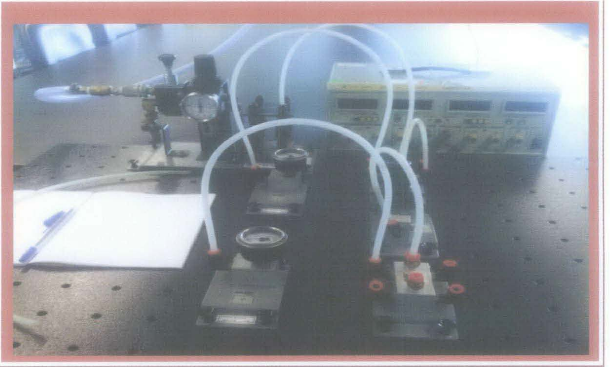
Figure 2.1.5.1 : Fuel Pressure system being test at Mechatronic Lab
