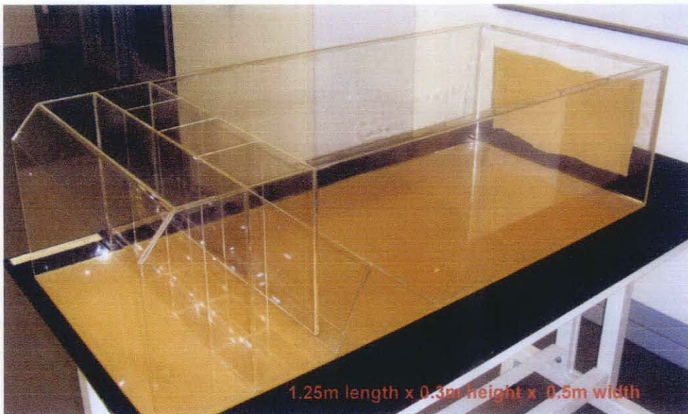
Figure 20: Water Container after finished fabrication
