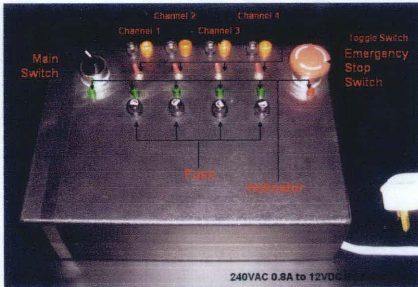
Figure 28: User Interface of Power Distribution System
