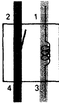
Figure 9: Two circuits in a four pin relay
