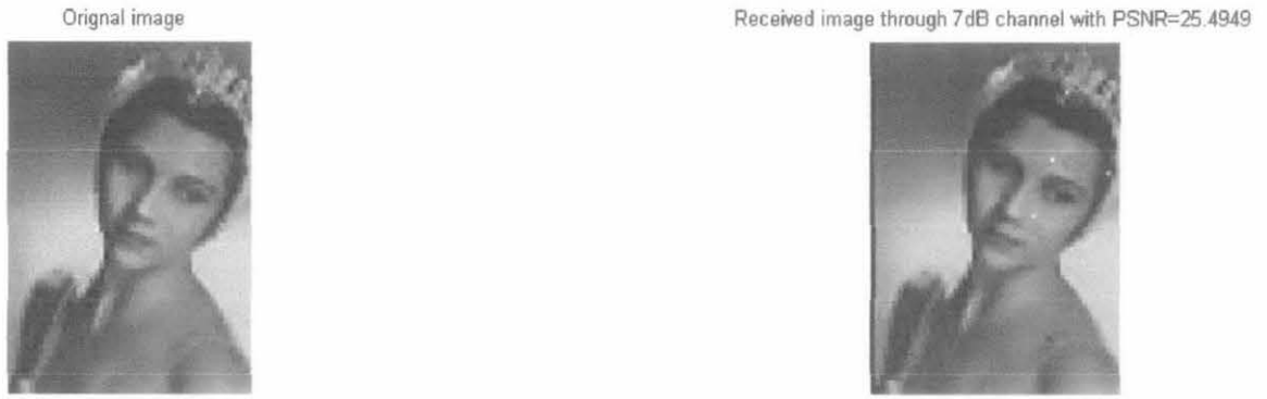
Figure 14: Original and received image of BCH code at 7 dB noise channel
