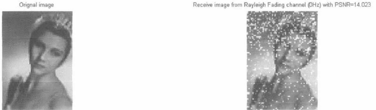
Figure 15: Image comparison for LDPC code in Rayleigh Fading Channel
