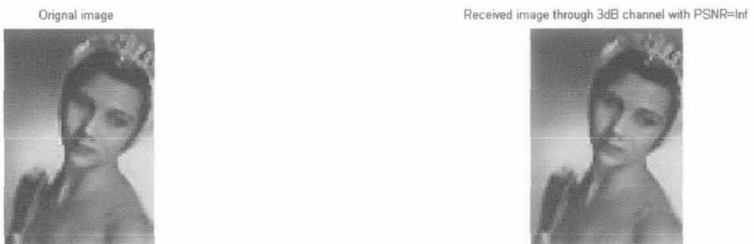
Figure 5: Original and received image of LDPC code at 3 dB noise channel
