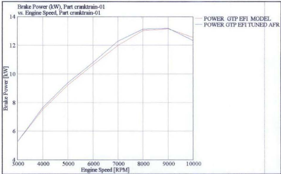
Figure 4.9: AFR Tuning of EFI System-Power Comparison
