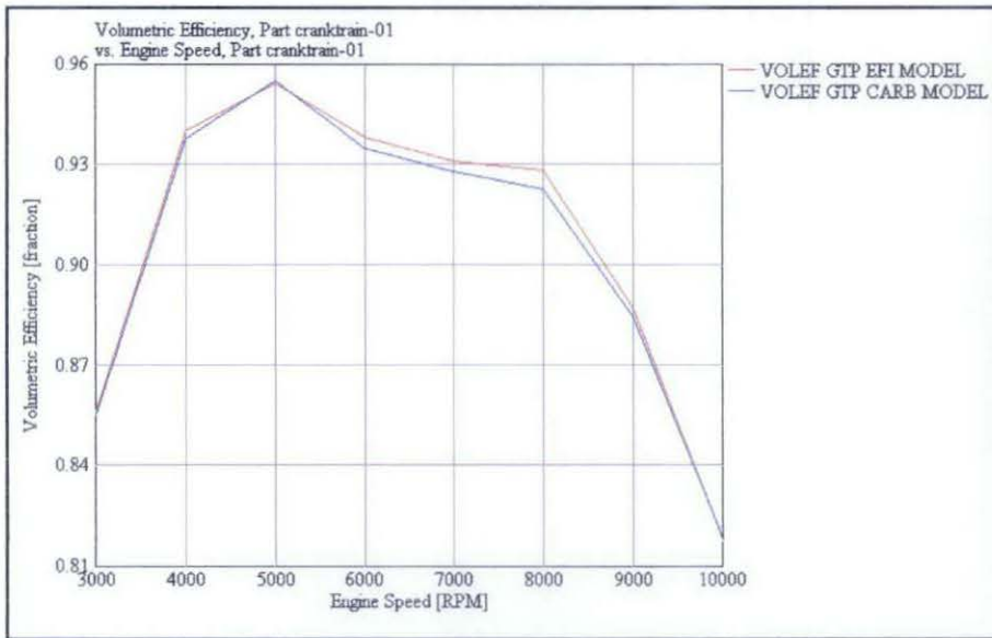
Figure 4.7 : Conversion-Volumetric Efficiency Comparison
