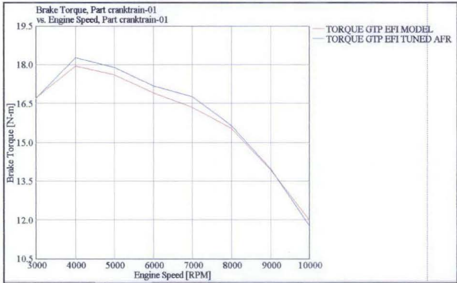
Figure 4.10: AFR Tuning of EFI System-Torque Comparison
