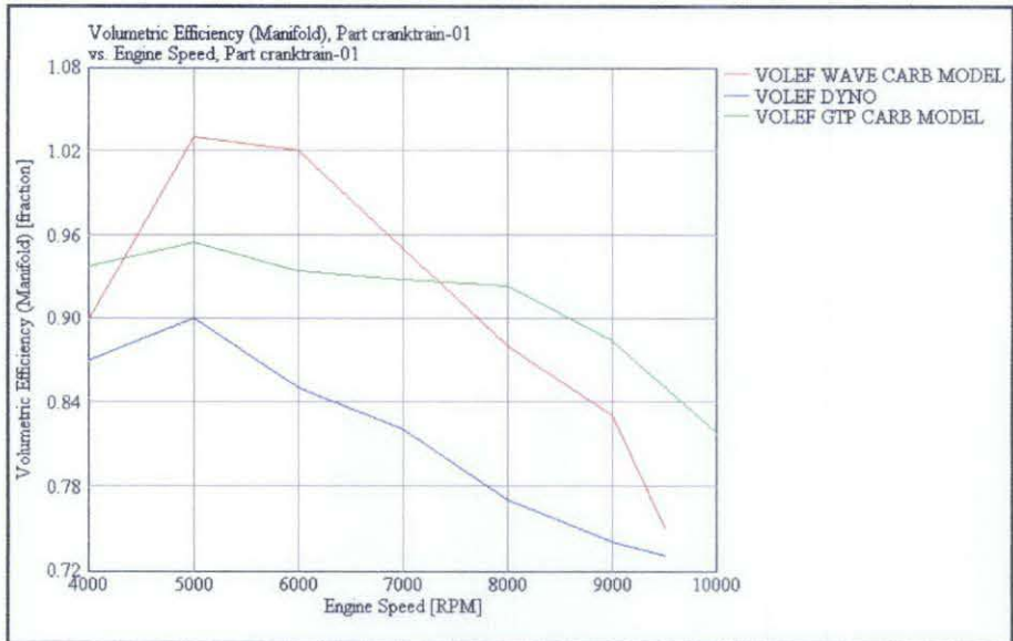
Figure 4.3 : Volumetric Efficiency Validation
