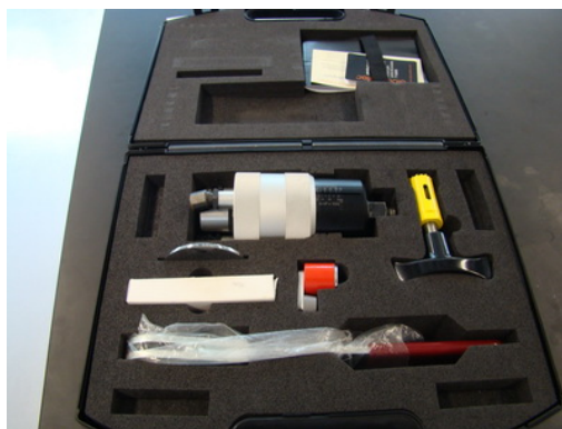
Figure L: The Full Kits of Pull off Adhesion or Dolly Test
