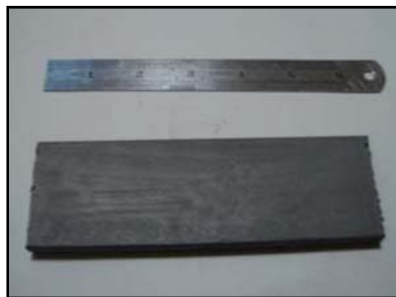
Figure 2.8: Zinc-Rich Epoxy Primer Coat on the Sample of ASTM-A36 Carbon Steel Structural Plate
