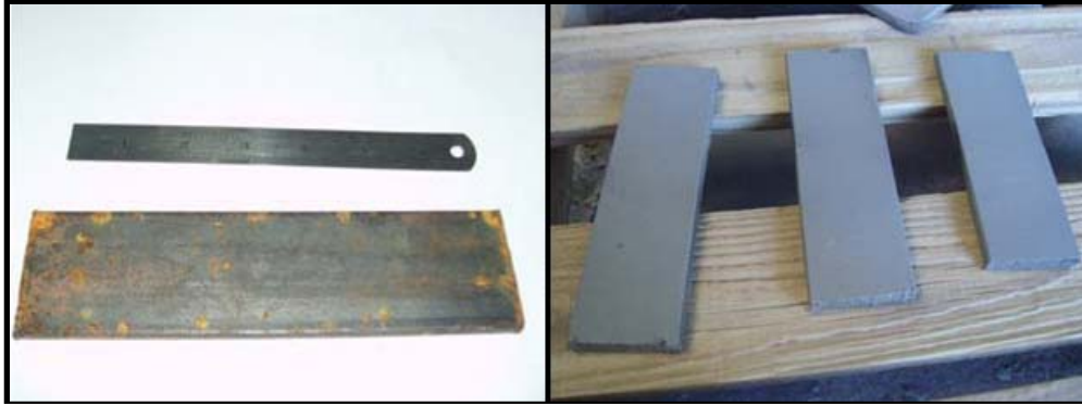
Figure 2.6: From Left - The Sample of ASTM-A36 Carbon Steel Structural Plate before and after blasting process respectively
