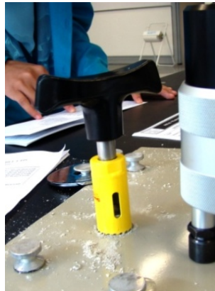
Figure 3.9: Special Coating Cutter to cut around the dolly down to the substrate
