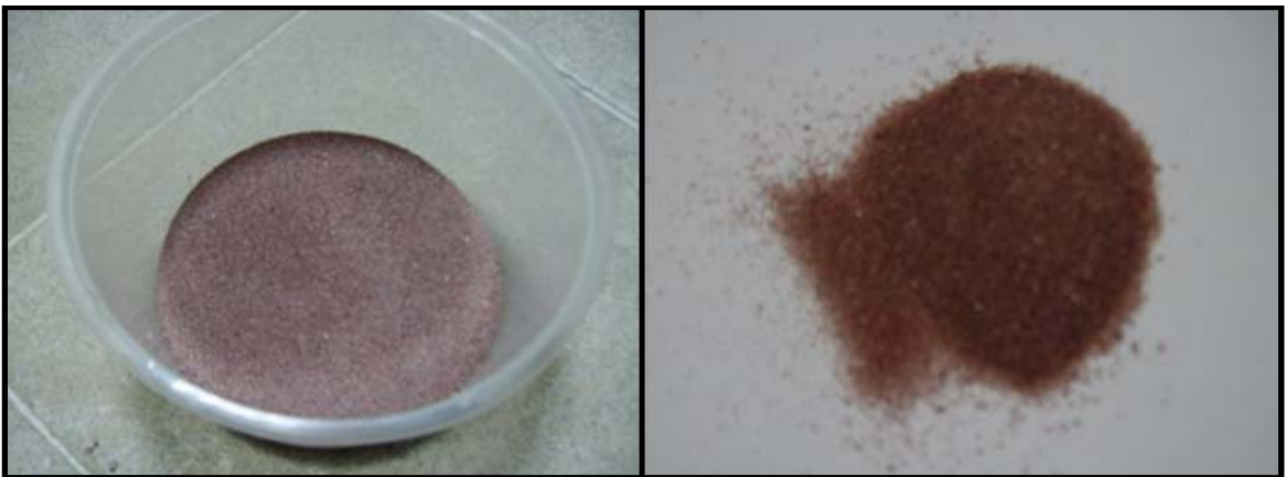
Figure 2.5: Metallic Abrasive GMA (Garnet Mineral Australia) type – (These samples were getting from one of the oil and gas services company in Malaysia)
