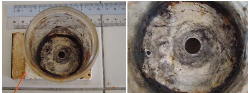
Figure 4.7: The effect of cathodic disbondment test on the drilled coated plate
