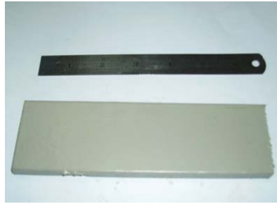
Figure 2.9: High-Solid Epoxy Mid-Coat (Second Coat) on the Sample of ASTM-A36 Carbon Steel Structural Plate
