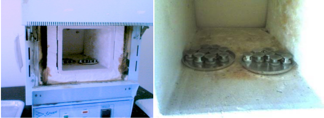
Figure J: Dollies were left in Furnace for two days before continue with the Pull-Off Adhesion Test
