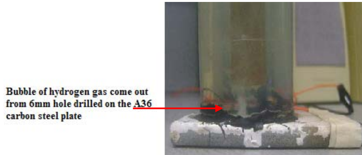
Figure 4.6: Bubble of Hydrogen Gas from Drilled Hole
