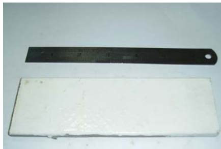
Figure 2.10: Top-Coat (Finish/Final Coat) on the Sample of ASTM-A36 Carbon Steel Structural Plate
