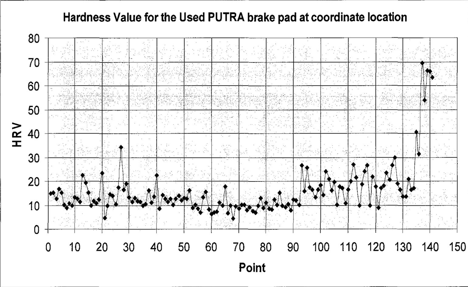
**Graph 4.2: Hardness Value for used PUTRA LRT Brake Pad in Coordinate location**
