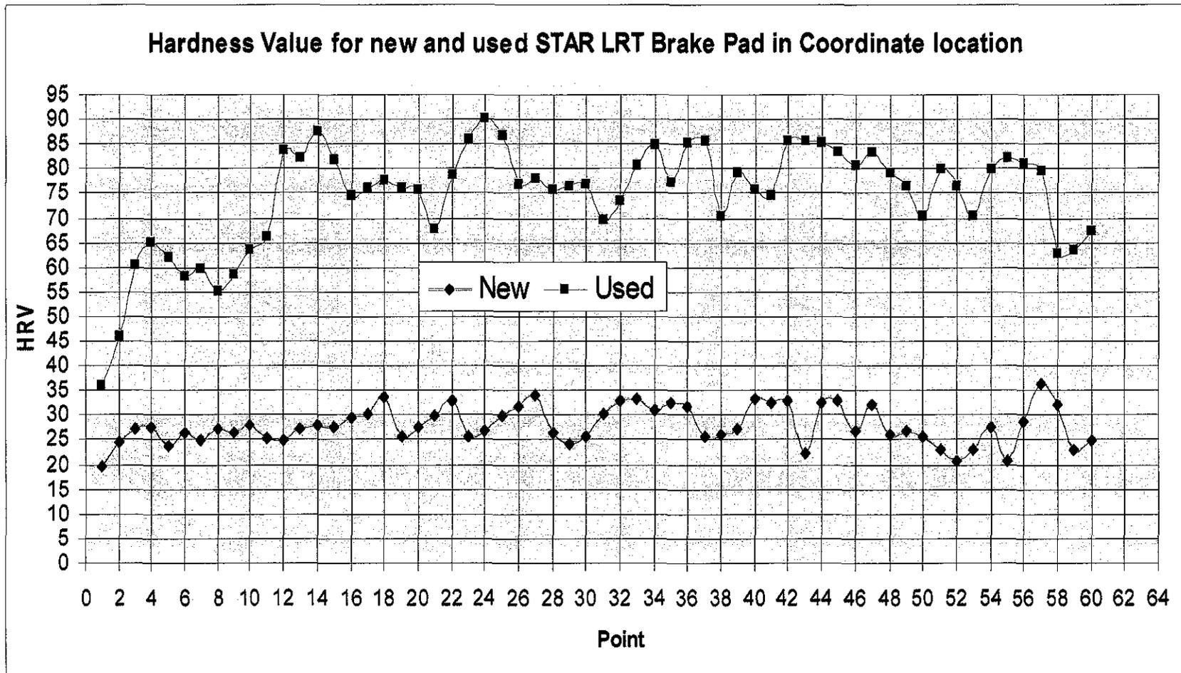
**Graph 4. 1: Hardness Value for new and used STAR LRT Brake Pad in Coordinate location**
