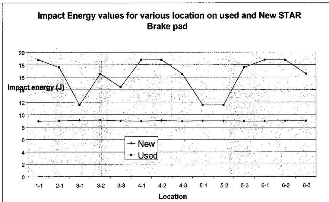
Graph 4.3: Impact Energy values for various location on used and New STAR Brake pad
