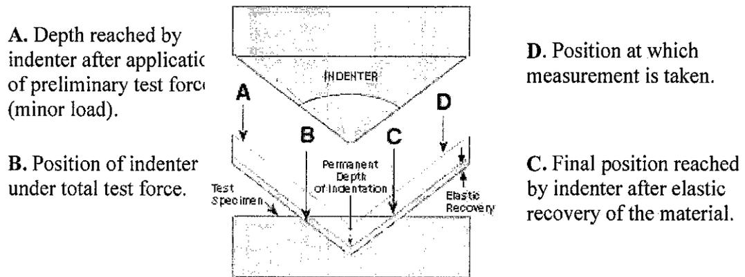
Figure 2.1: Rockwell measurement Principles
