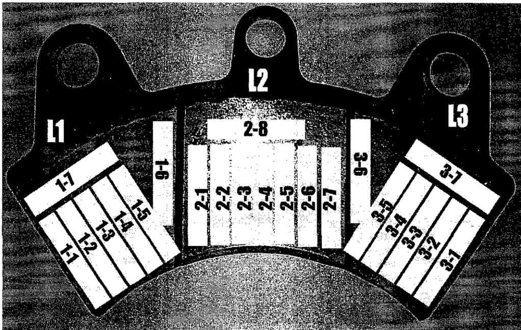
Figure 4.4: Impact test Location at PUTRA LRT Brake Pad
