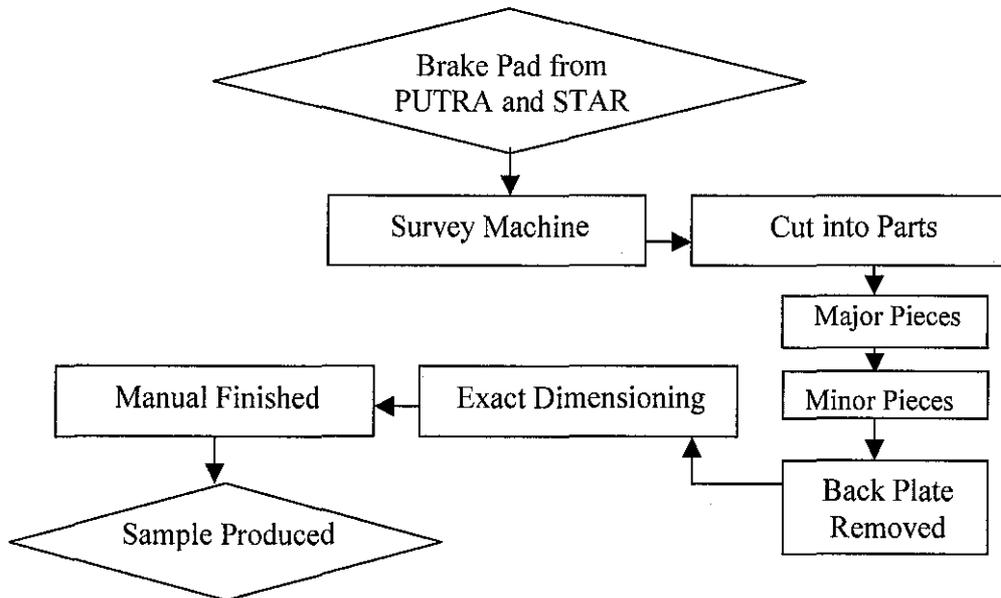
Figure 3.4: Flowchart of preparation for impact test sample.
