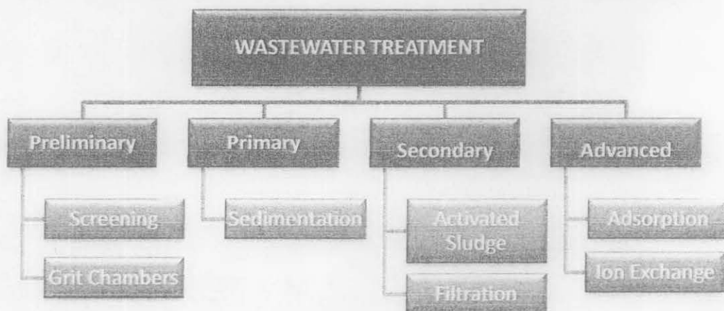
Figure 1: Wastewater treatment process
