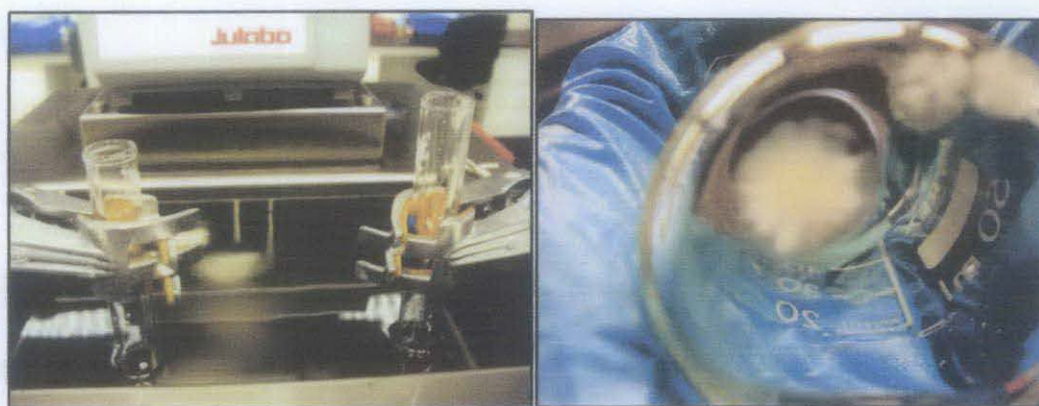
Figure 3.2: Sample of ionic liquid is cooled down to crystallization temperature in ethylene glycol bath at cooling rate of 1°C /min. Seed crystal is used to induce crystallization.
