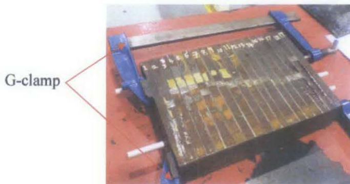
Figure 3.22: The assembled laminates with G-clamp on both sides
