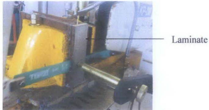
Figure 3.15: The coolant running through the laminate
