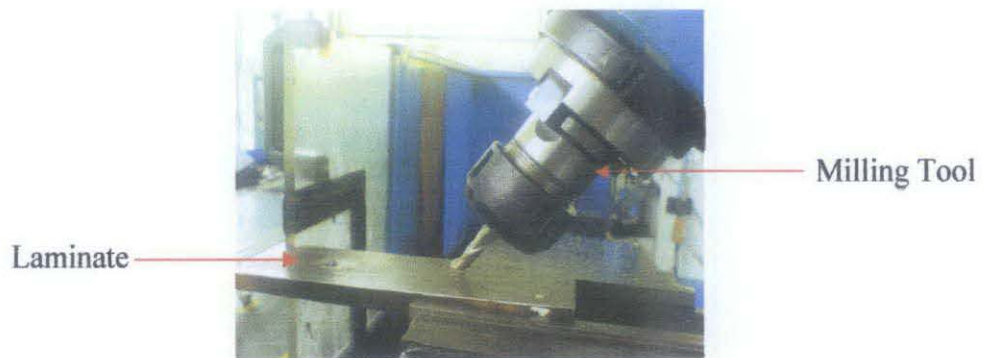
Figure 3.18: Angle drilling by milling machine
