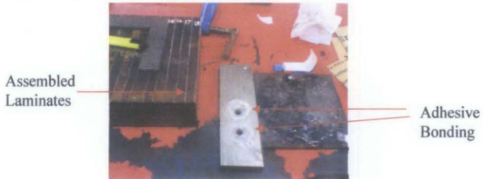
Figure 3.21: Adhesive bonding on the laminate
