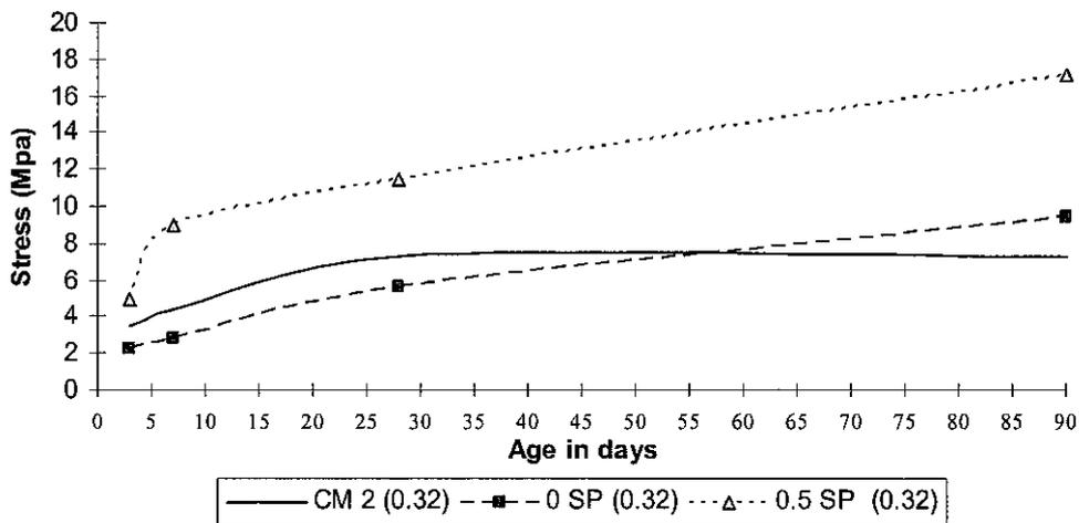
Figure 15: Compressive strength results for 0.32 w/c.
