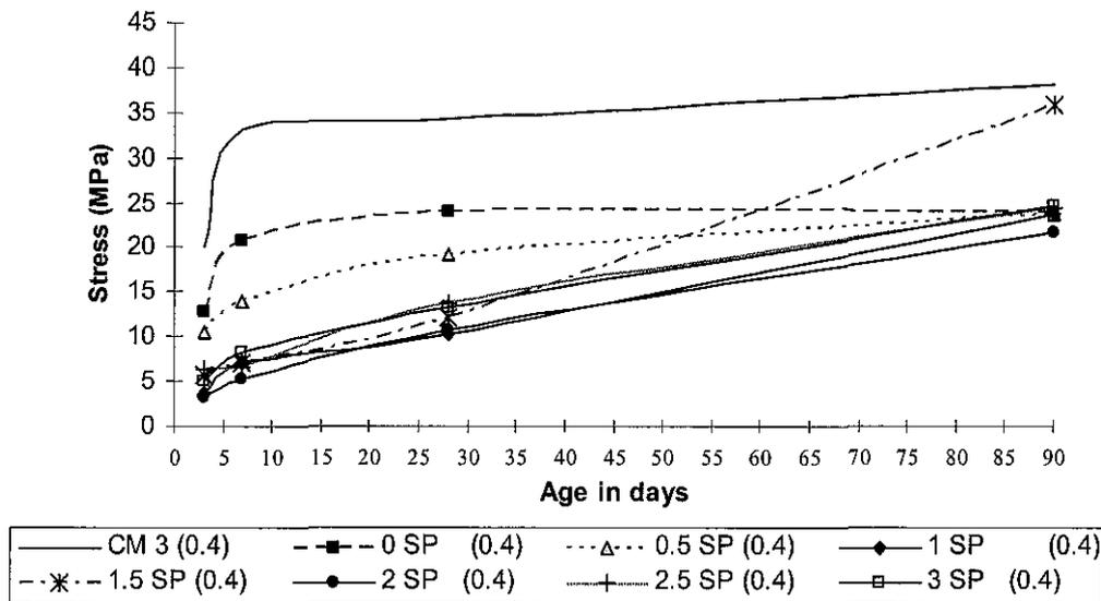
Figure 16: Compressive strength results for 0.4 w/c.
