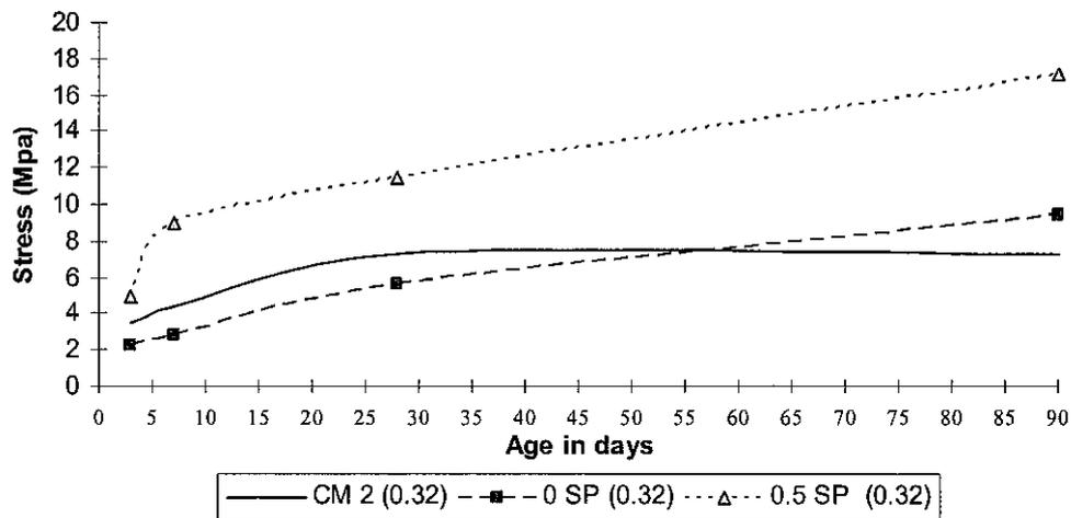
Figure 15: Compressive strength results for 0.32 w/c.
