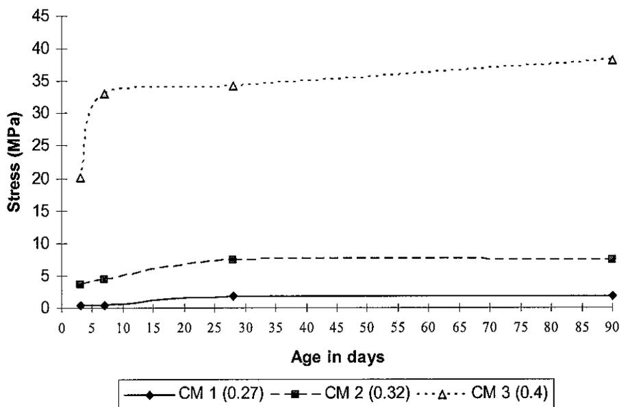
Figure 14: Compressive strength results for Control Mix.
