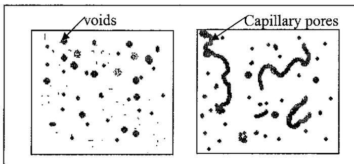
*Figure 19: Comparison of pores distribution and connectivity between two same porous samples.*
