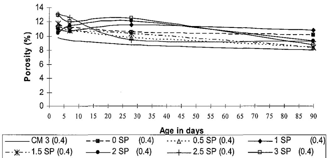
Figure 17: Porosity results for 0.4 w/c.
