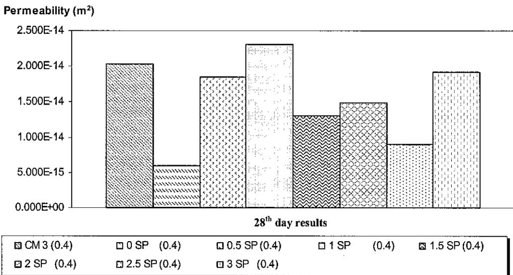
Figure 18: Permeability test results for 0.4 w/c.
