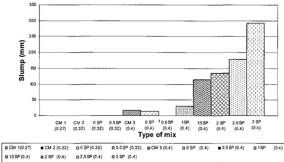
Figure 5 : Slump results for all mix.
