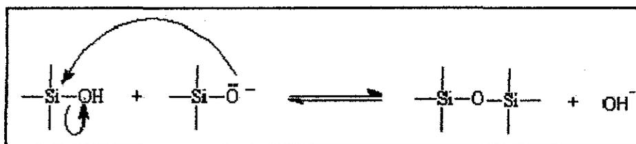
Figure 2.4: Nucleophilic Attack to Form Siloxane Bond
