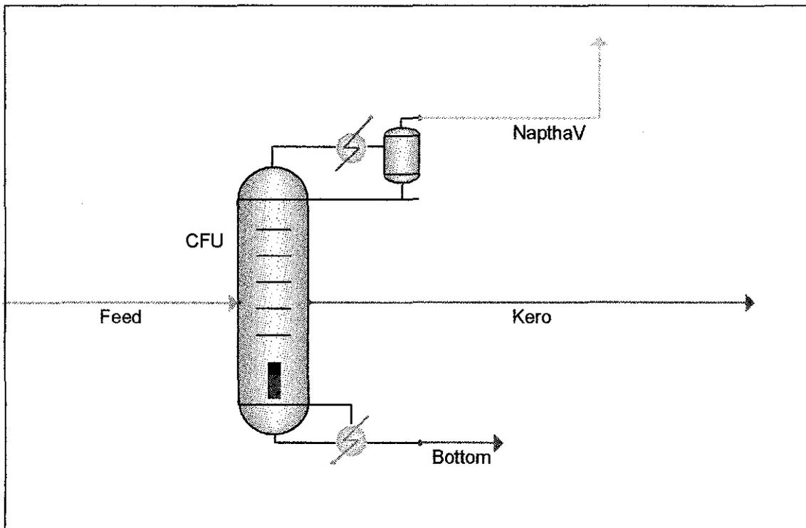
Figure 4: Light End Unit Developed in iCON
