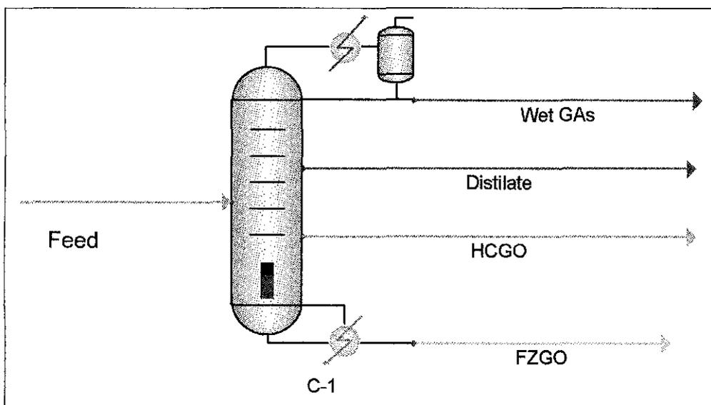
Figure 5: Delayed Coker Unit Model Developed in iCON
