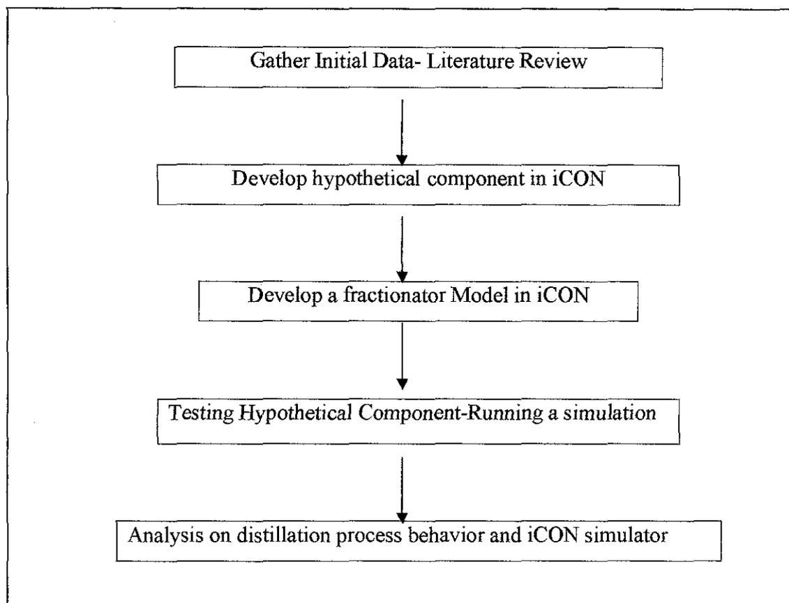
Figure 2 : Thermal Data Extraction Procedure
