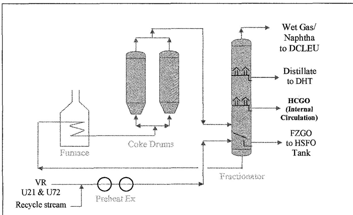
Figure 1: Overview of Delayed Coker Unit/Coking Section
